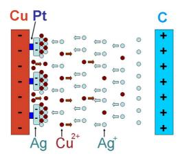
A scheme of the electrochemical process for Ag deposition
