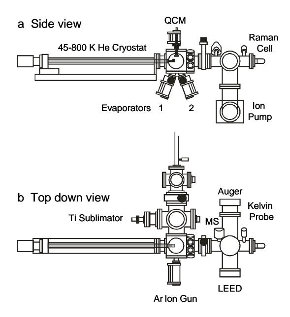
**Figure S1.** a) Side view and b) top view of custom-built UHV Raman system consisting of deposition and analysis chambers separated by 6" gate valve and linearly-translatable cryogenic sample arm.
