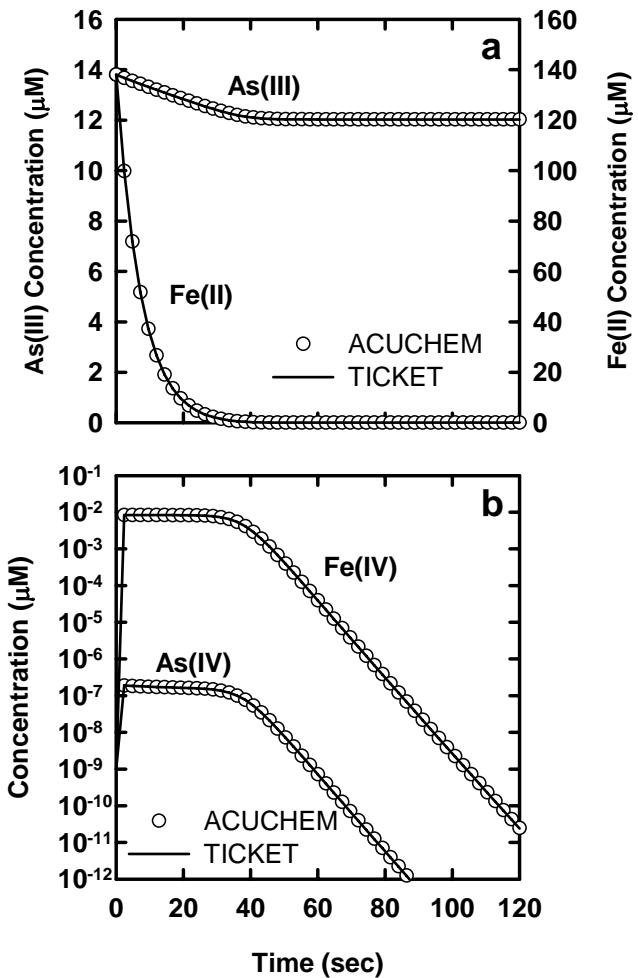
**Figure S2.** Comparison of TICKET and ACUCHEM (8) model results for Fe(II)-catalyzed oxidation of As(III) in batch systems at fixed dissolved oxygen concentration and pH of 250  $\mu\text{M}$  and 8.0, respectively.
