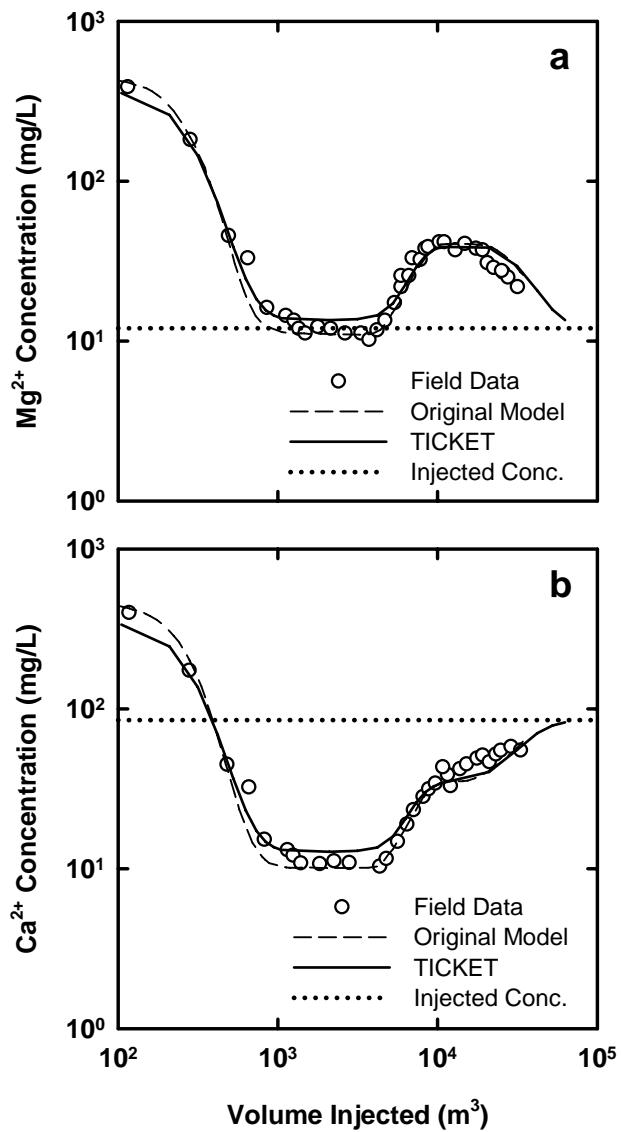
**Figure S1.** Comparison of TICKET-calculated breakthrough curve for (a) Mg<sup>2+</sup> and (b) Ca<sup>2+</sup> with field data and model results of Valocchi et al. (1).
