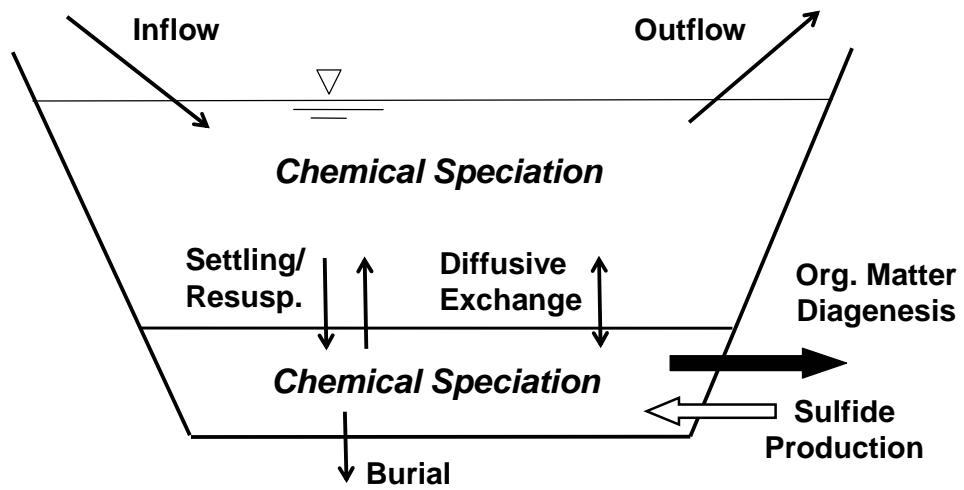
**Figure S3.** Modeling framework for metal cycling in an idealized lake.
