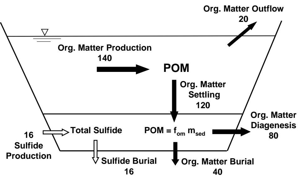
**Figure S4.** Average annual organic matter and sulfide cycles in lake.
