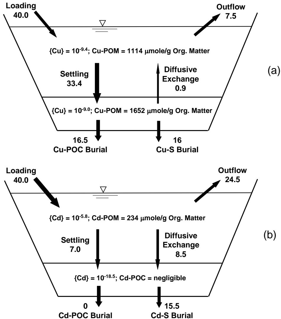
**Figure S5.** Steady-state concentrations and fluxes for copper (a) and (b) cadmium in a circumneutral, soft water lake. (Metal flux rates, as depicted by arrows on the diagrams above, are given in mmoles / m<sup>2</sup> / yr.)
