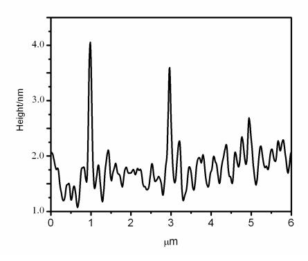
**Figure S1.** Height profile of OPA line arrays generated by DPN at writing speeds of 0.04, 0.16, and 0.64  $\mu$ m/sec (from left to right). The height profile was obtained from the topography AFM image shown in Figure 1B.
