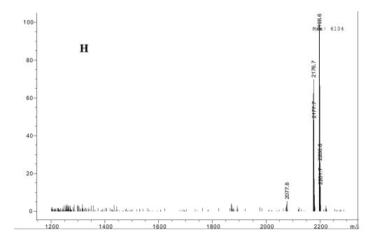
**H**: ESI-MS (API, positive ion mode) of Por-PEG<sub>4</sub> (parent peak at 2176 and Na<sup>+</sup> adduct 2198)
