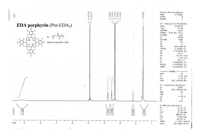
K: 500 MHz <sup>1</sup>H NMR (CD<sub>3</sub>OD) of Por-EDA<sub>4</sub>
