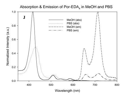
**J**: Absorption and emission of Por-EDA<sub>4</sub> in methanol and PBS. Note the shifts in absorption in the aqueous media.
