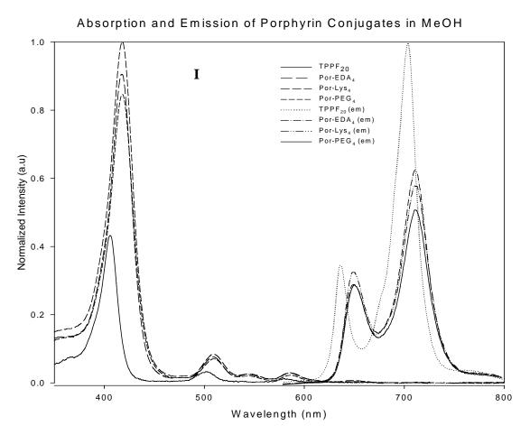
**I:** Absorption and emission of the parent porphyrin  $(TPPF_{20})$  and the derivatives (Por-EDA<sub>4</sub>, Por-Lys<sub>4</sub>, Por-PEG<sub>4</sub>) in MeOH.
