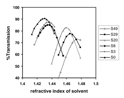
Index matching data for determination of refractive index of spheres. The refractive index of the solvent mixture was determined using an Abbe refractometer. Lines are guides to the eye only.
