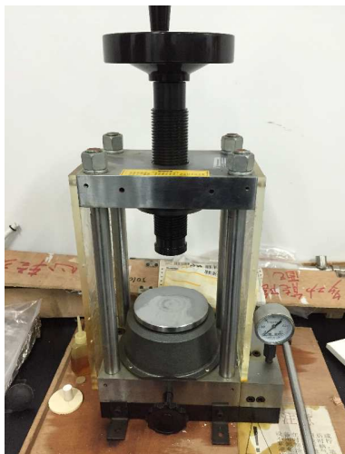
Fig. S3 The press machine used to fabricate membrane green compacts.
