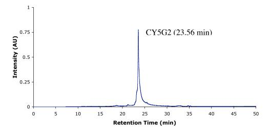
RP-HPLC conditions: Solvent A: 0.004% TFA in water, Solvent B: 0.004% TFA in acetonitrile, C18 analytical column, Vydac, 218TP54, flow rate 1 ml/min. 100% solvent A to 100% solvent B in 50 min.
