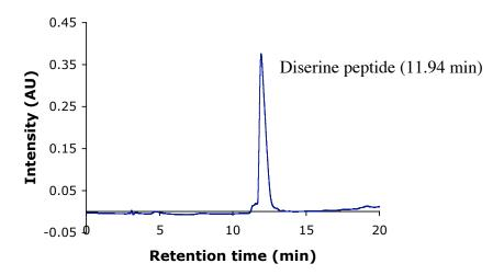
RP-HPLC conditions: Solvent A: 0.1% TFA in water, solvent B: 0.1% TFA in acetonitrile, C18 analytical column, Vydac, 218TP54, flow rate 1 ml/min. 100% solvent A to 100% solvent B in 50 min.
