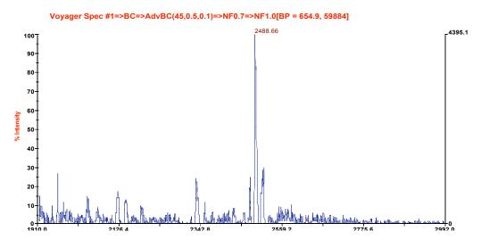
MALDI-TOF conditions: Instrument: Voyager-DE PRO (PerSeptive Biosystems), Instrument mode: Negative, VOLTAGES: Accelerating: 20000, Grid: 95, Guide Wire: 0.05, Delay Time: 100 nsec. NOTE: Partial cleavage of the hydrazone linkage was observed under MALDI conditions (alpha-cyano-4-hydroxycinnamic acid as a matrix and 0.1% trifuoroacetic acid in 50% acetonitrile) homogeneity and purity of CY5G2 was confirmed using RP-HPLC (see below)
