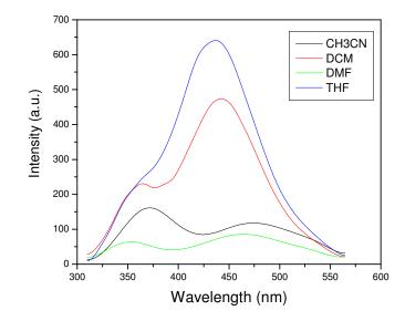
**Figure S3**. Fluorescence spectra of **2** (concentration  $1 \times 10^{-6}$  M) in different solvent (PERKIN ELMER, LS50B, Luminescence Spectrometer)
