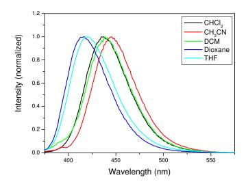
Figure S2. Fluorescence spectra of 1 (concentration  $1 \times 10^{-6}$  M) in different solvent (PERKIN ELMER, LS50B, Luminescence Spectrometer)
