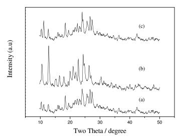
**Figure S6**: X-ray powder diffraction spectra of compound **1**: (a) hydrated condition (b) de-hydrated upon heating at 110 °C for 1 h and (c) re-hydrated condition.
