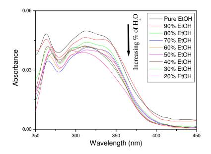
**Figure S4**. Uv-Vis spectra of compound **1** in different ratio (v/v) of water/ethanol mixture (JASCO, V-570, UV/VIS/NIR/ Spectrophotometer).
