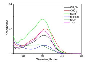
**Figure S1**. UV-Vis spectra of compound **1** (concentration  $1 \times 10^{-5}$  M) in different solvent (JASCO, V-570, UV/VIS/NIR/ Spectrophotometer)
