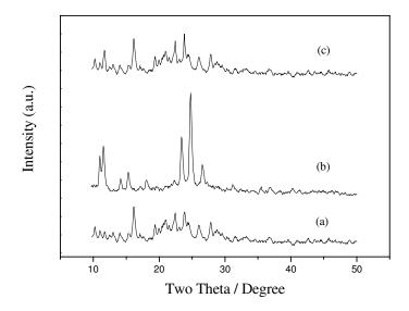
**Figure S7:** X-ray powder diffraction spectra of compound **2**: (a) hydrated condition (b) de-hydrated upon heating at 100 °C for 1 h and (c) re-hydrated condition.
