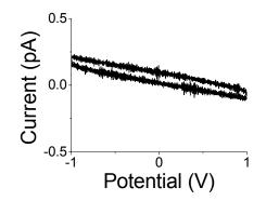
**Figure 2.** Cyclic voltammogram recorded in a solution containing 10 mM  $IrCl_6^{3-}$  and 0.1 M KNO<sub>3</sub> at a scan rate of 20 mV s<sup>-1</sup>, using a silicon AFM probe (FESP, L. O. T. –Oriel Gmbh & Co.) which had been thermally oxidised for 3 hours by the procedure described above, as the working electrode. An Ag/AgCl reference electrode was employed.
