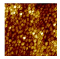
Figure 3. 1 µm square height image of Au on a silicon substrate (15 nm height scale).
