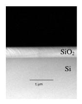
Figure 1. FE-SEM cross-section image of a thermally oxidised silicon AFM probe.
