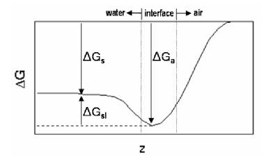
**Figure 1S.** Schematic diagram of a free energy profile for transferring a gas phase molecule accross the air/water interface. The interfacial region is indicated by the dotted lines.  $\Delta$ Gs denotes the free energy of solvation,  $\Delta$ Ga the free energy of adsorption on the water surface, and  $\Delta$ Gsl the free energy difference associated with moving the solute from the surface into the bulk.
