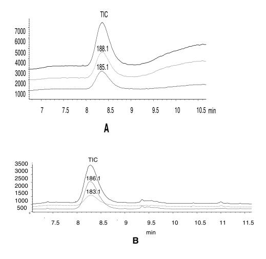
Mass Spectra of Detection of <sup>18</sup>O-Labeled Spirodihydantoin with Spirodihydantoin and Labeled Spirodihydantoin as Internal Standards
