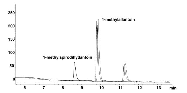
Oxidation of N9-Methyluric Acid (dotted line: without spiking of 1-methylSpd; solid line: with spiking of 1-methylSpd)
