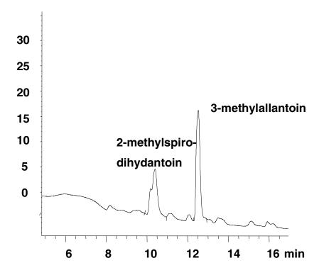
Selective Ion Monitoring Chromatograms of Detection of Spirodihydantoin with Labeled Spirodihydantoin as Internal Standard (A: positive ion mode; B: negative ion mode).
