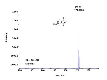
2-Methylspirodihydantoin from oxidation of N7-methyluric acid or decomposition of 5-CI-N7methylisouric acid
