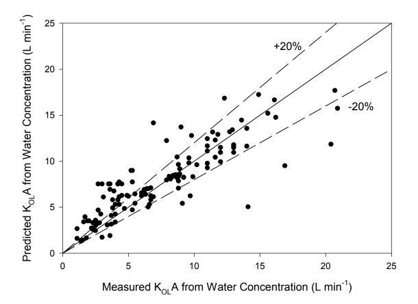
Figure S4. Predicted versus measured values of the overall mass transfer coefficient for shower
