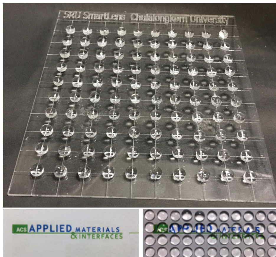
Figure S8 A set of 100 ePDMS planoconvex lenses (5-mm diameter) fabricated by the confined sessile drop technique and their optical effect when placed on printed characters.
