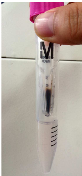
Fig.S4 The picture of RC -BSA NPs concentrated aqueous after crosslinking using a 100 kDa filter at 6000 rpm for 20 min with a nearly colorless filtrate
