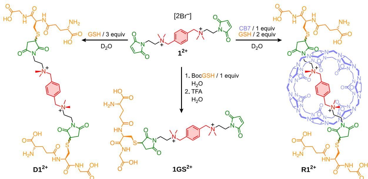
**Scheme S2.** Synthesis of *p*-xylylene-bisaminium dumbbell  $D1^{2+}$ , semidumbbell  $1GS^{2+}$ , and the corresponding CB7 [2]rotaxane  $R1^{2+}$ , from the bis(maleimide)  $1^{2+}$ .
