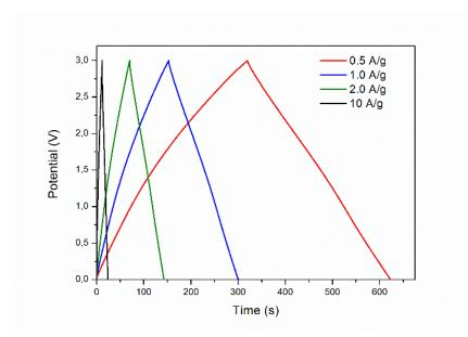
**Figure S3.** Galvanostatic charge-discharge at different current densities using NDMC-10 with EMIMBF<sub>4</sub> as electrolyte.
