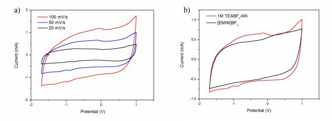
**Figure S4.** Electrochemical measurements of NDMC-10 in a 3-electrode cell: (a) Cyclic voltammetry of NDMC-10 in organic electrolyte at different scan rates (b) Cyclic voltammetry of both organic and ionic liquid electrolytes at 50 mV/s.
