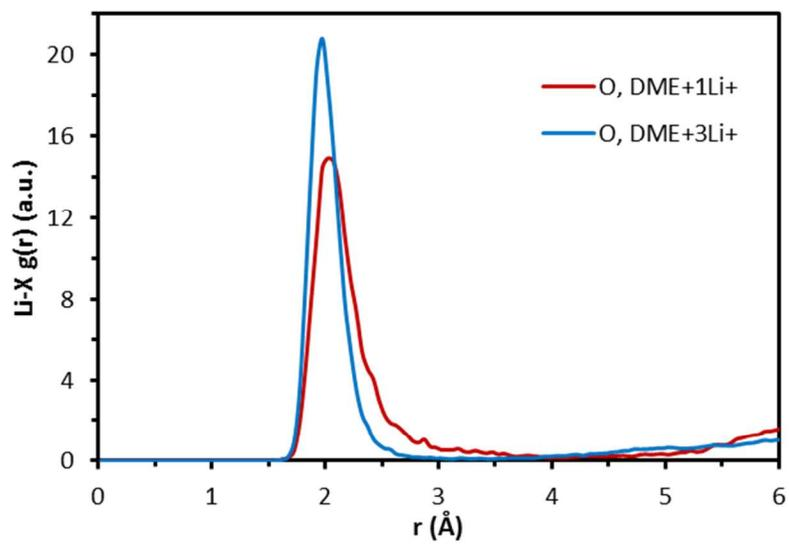
**Figure S 18.** Radial distribution function for Li<sup>+</sup>--X (X=O and F atoms) pairs for pure DME with one and three additional ions.
