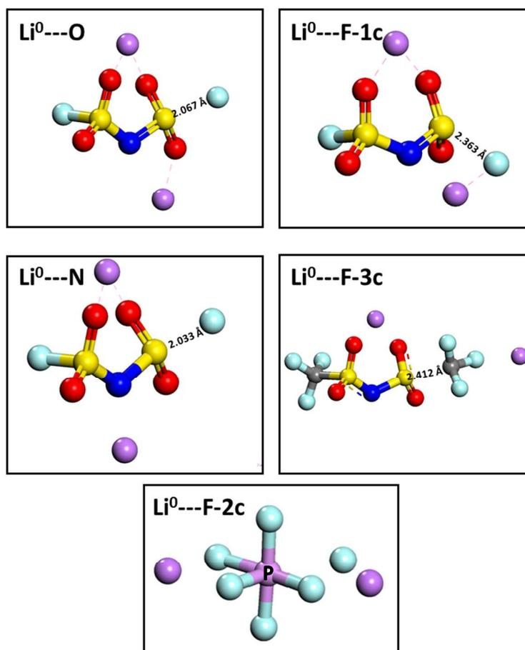
**Figure S13.** Resulting optimized configurations formed from spontaneous reactions caused by  $\text{Li}^0$  radical attack. Color code as in Figure 1.
