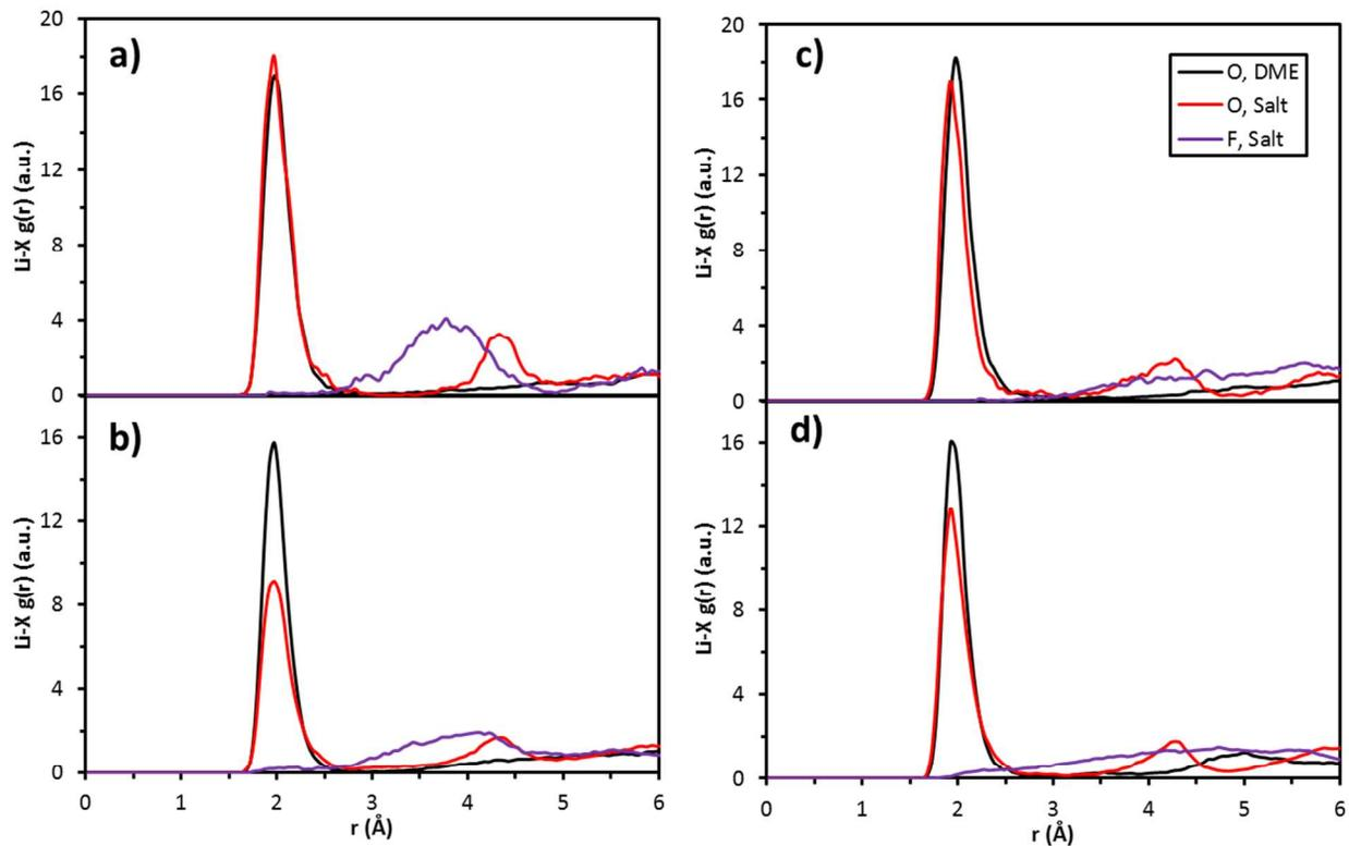
**Figure S16.** Radial distribution function for  $\text{Li}^+-\text{X}$  ( $\text{X}=\text{O}$  and  $\text{F}$  atoms) pairs for solutions with one additional cation. a) 1M-LiFSI, b) 4M-LiFSI, c) 1M-LiTFSI, and d) 4M-LiTFSI.
