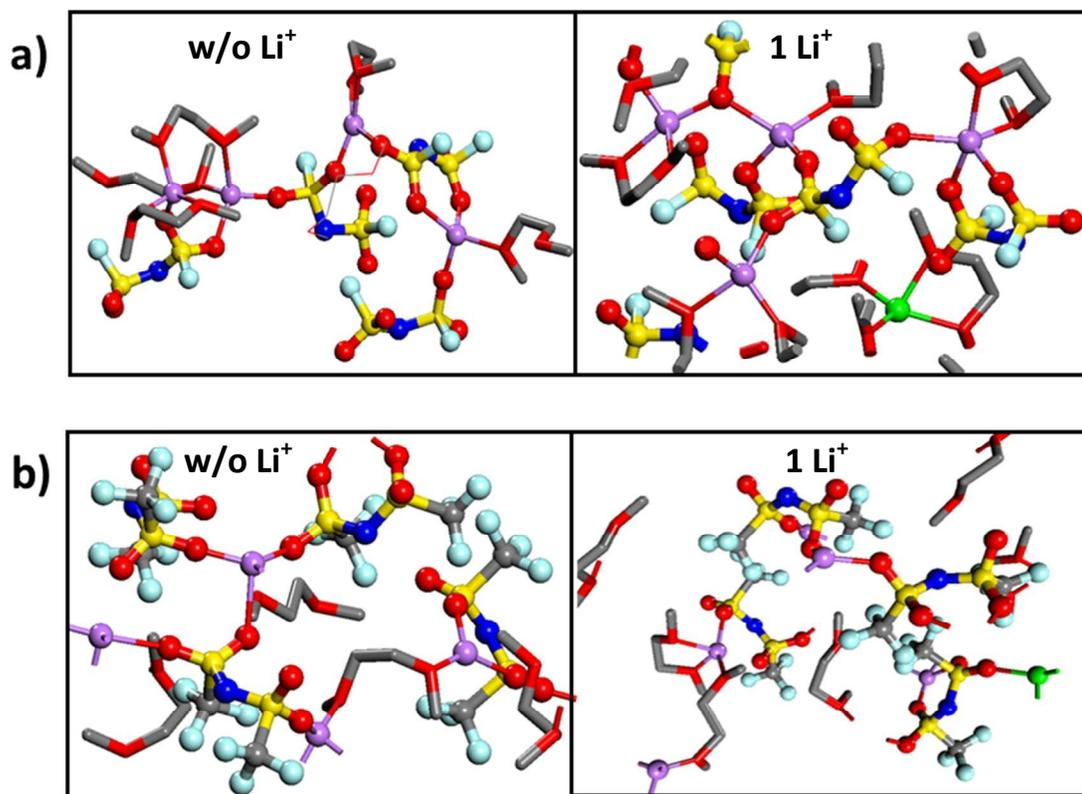
**Figure S14.** 4M-salt electrolyte solutions after 20ps of simulation time at 330K with different concentration of Li-ions. a) LiFSI and b) LiTFSI, respectively. Color code as in Figure 8. Hydrogen atoms are not shown for clarity.
