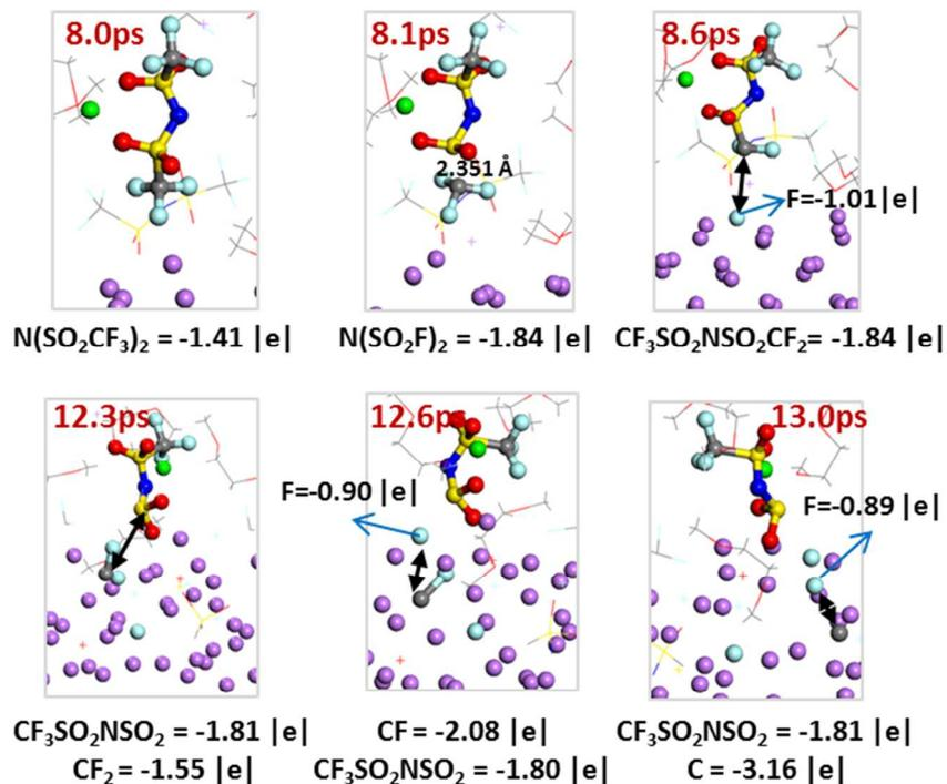
**Figure S7.** 2-LiTFSI reduction mechanism in a 4M-LiTFSI/DME solution. Average charge of Li (form LiTFSI) 0.88 ( $\pm 0.01$ ) |e| over the entire simulation time. Color code as in Figure 1.
