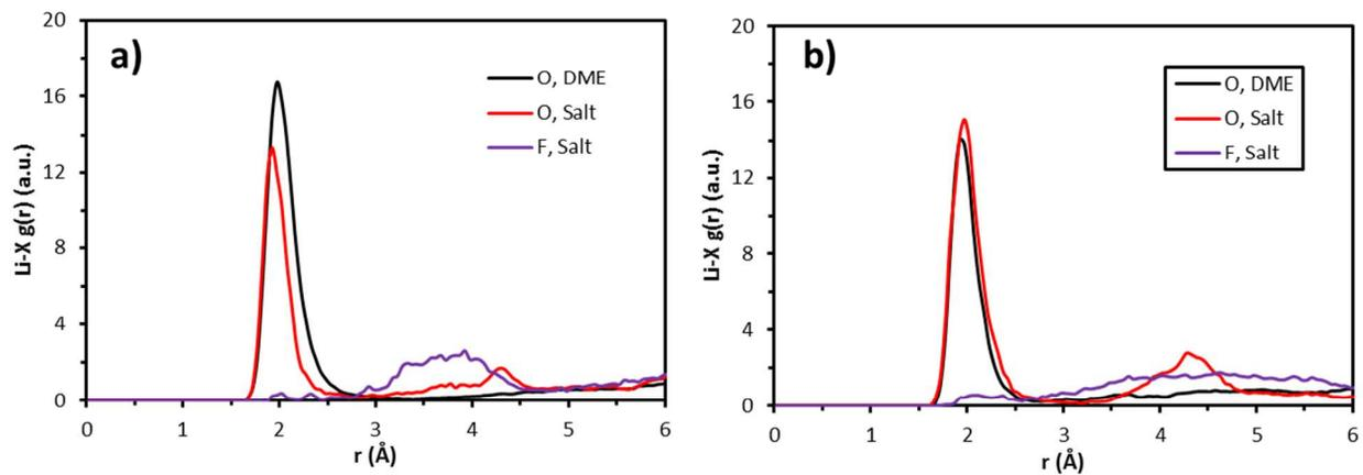
**Figure S17.** Radial distribution function for  $\text{Li}^+-\text{X}$  ( $\text{X}=\text{O}$  and  $\text{F}$  atoms) pairs for solutions with three additional ions. a) 1M-LiFSI, and b) 1M-LiTFSI
