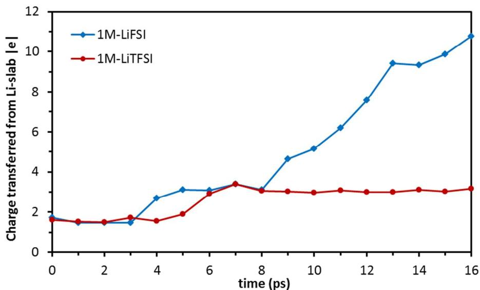
**Figure S3.** Total charge transfer from the Li anode to the electrolyte in 1M salt in DME. Non-zero initial charge ( $\sim 2$  |e|) is due to solvation/interaction of surface lithium atoms with the electrolyte from the initial model, see example in Figure S10b.
