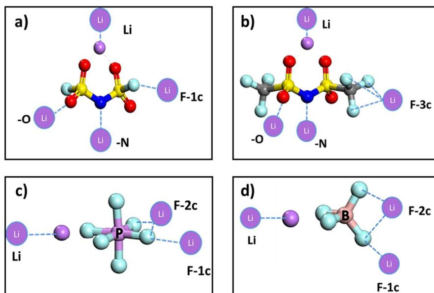
**Figure S12.** Initial configurations used for study of  $\text{Li}^x$  ( $x=0, 1$ ) attack to different salts: a) LiFSI, b) LiTFSI, c) LiPF<sub>6</sub>, and d) LiBF<sub>4</sub>. Color code as in Figure 1.
