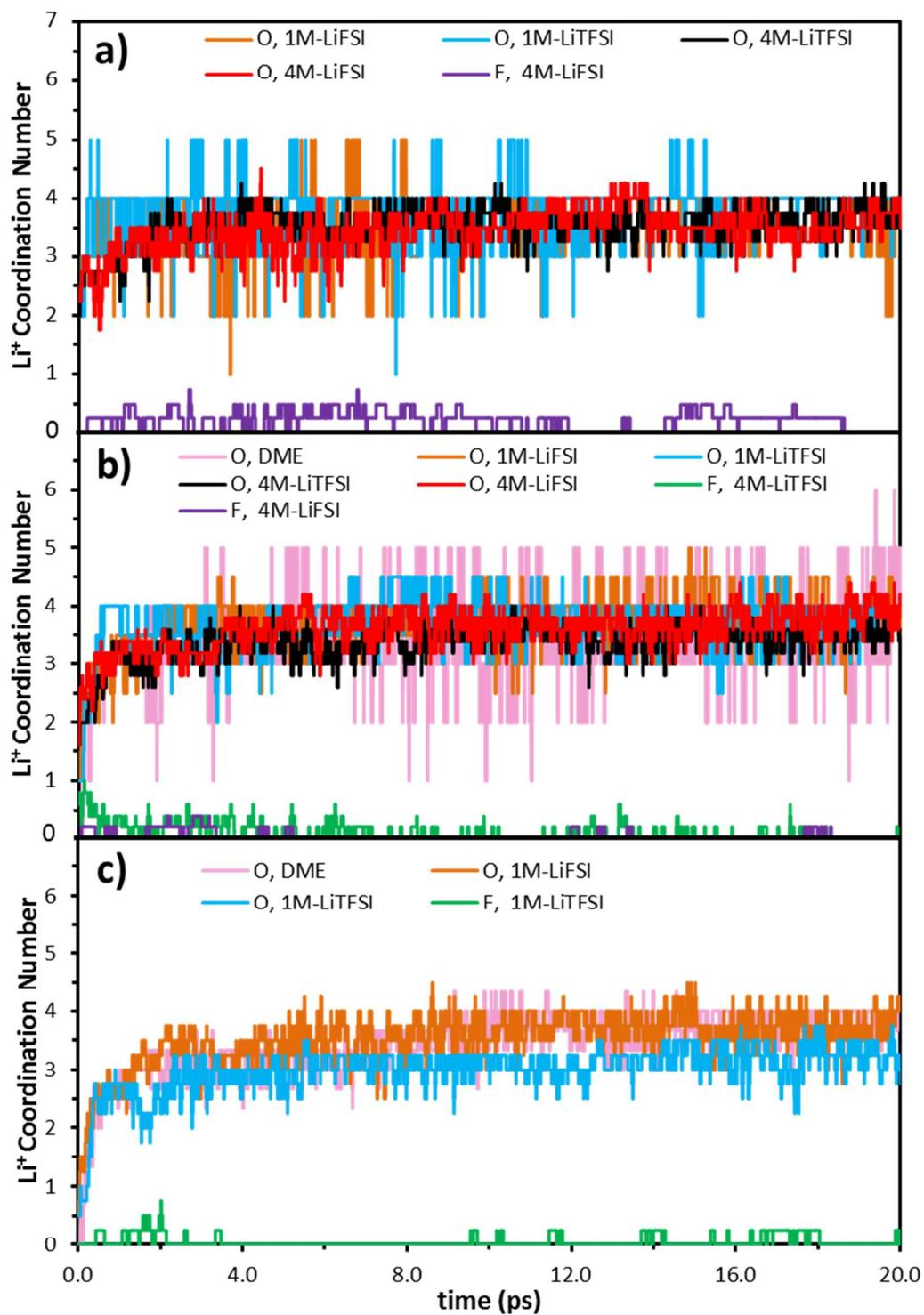
**Figure S19.** Average coordination numbers calculated as a function of time under different concentrations of lithium ions: a) w/o  $\text{Li}^+$ , b) 1  $\text{Li}^+$ , and c) 3  $\text{Li}^+$ .
