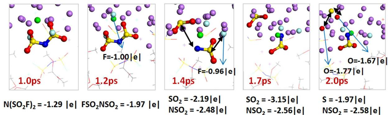
**Figure S4.** 2-LiFSI reduction mechanism in a 4M-LiFSI/DME solution. Average charge of Li (from LiFSI)  $0.83 (\pm 0.04)$  |e| over the entire simulation time. Color code as in Figure 1.
