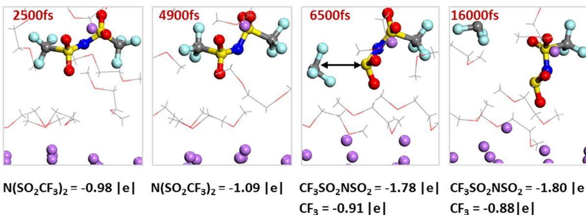
Figure S2. 1M-LiTFSI in DME reduction mechanism. Average charge of Li (from LiTFSI) is 0.88 (±0.01) |e| over the entire simulation time. Color code as in Figure 1.
