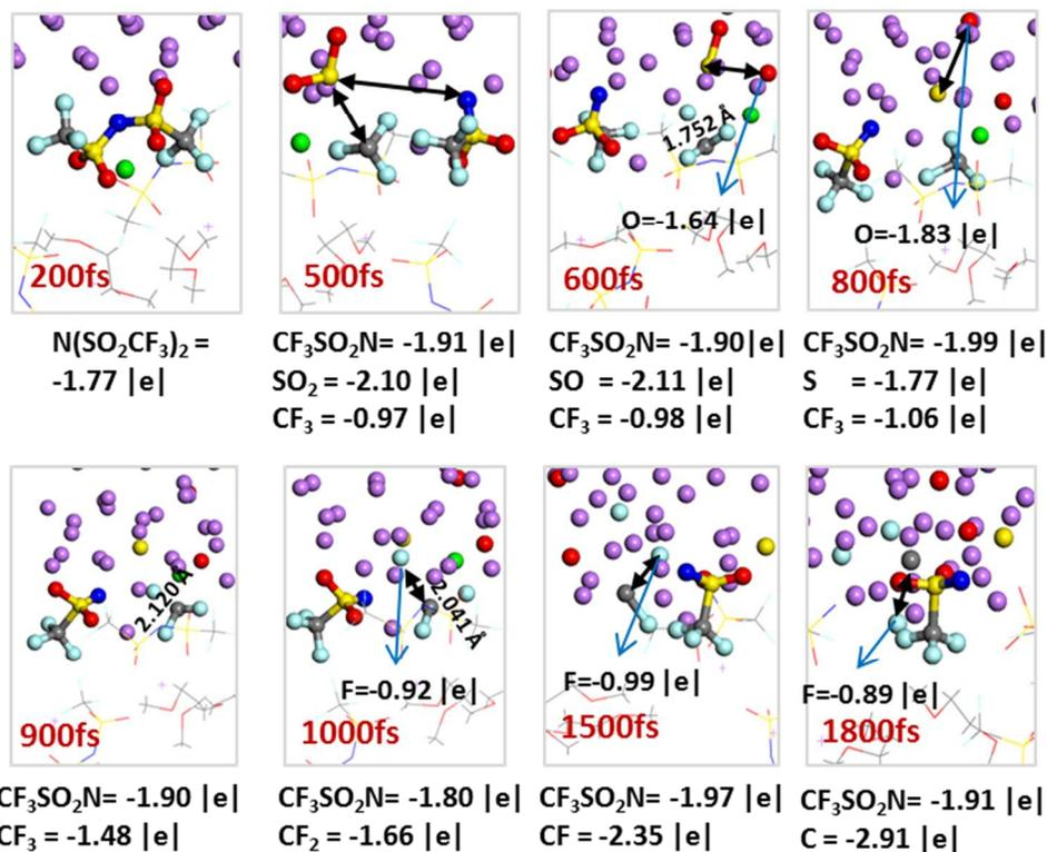
**Figure S8.** 3-LiTFSI reduction mechanism in a 4M-LiTFSI/DME solution. Average charge of Li (form LiTFSI) 0.85 ( $\pm 0.01$ ) |e| over the entire simulation time. Color code as in Figure 1.
