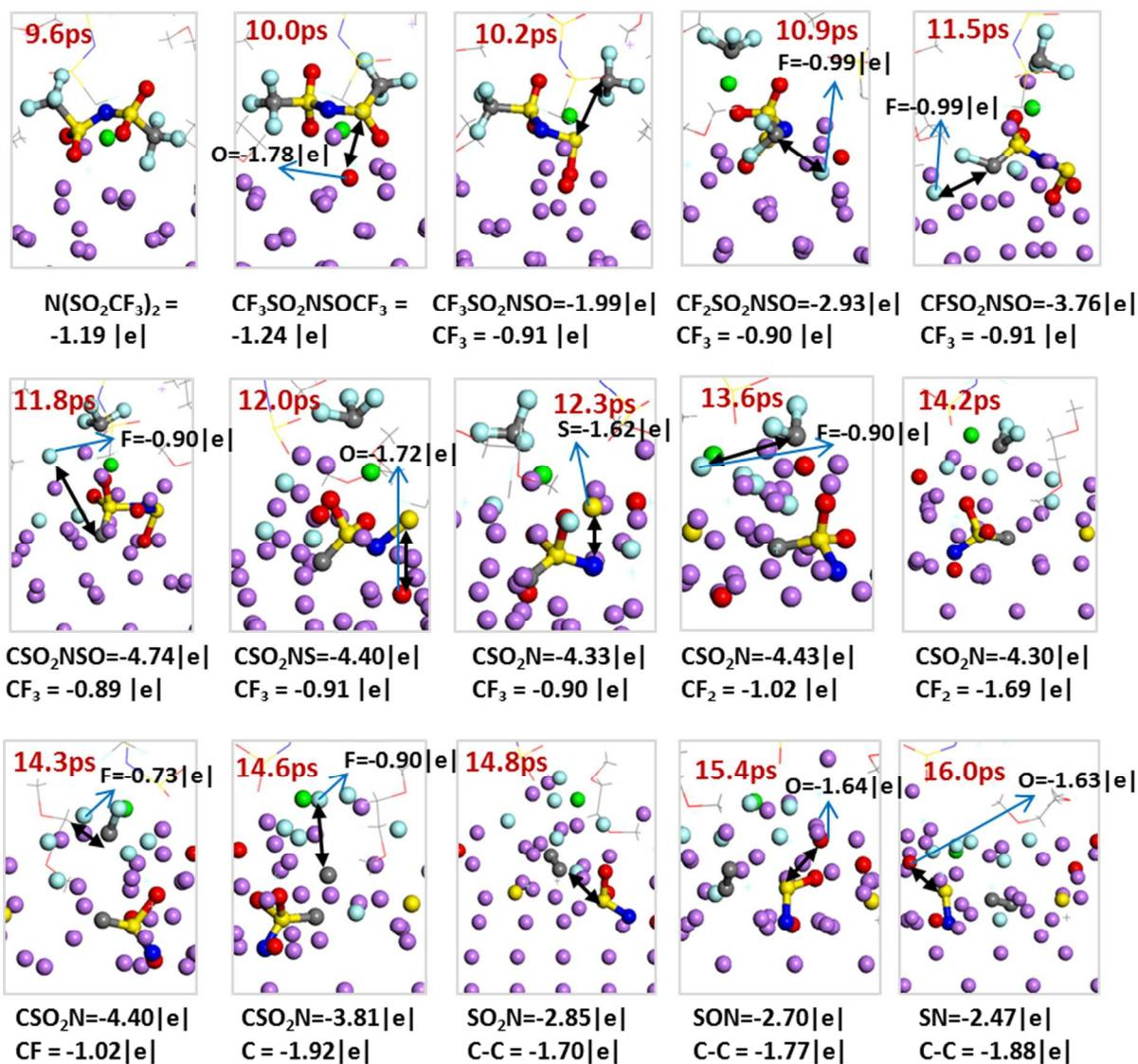
**Figure S9.** 4-LiTFSI reduction mechanism in a 4M-LiTFSI/DME solution. Average charge of Li (from LiTFSI)  $0.87 (\pm 0.03) |e|$  over the simulation entire time. Color code as in Figure 1.
