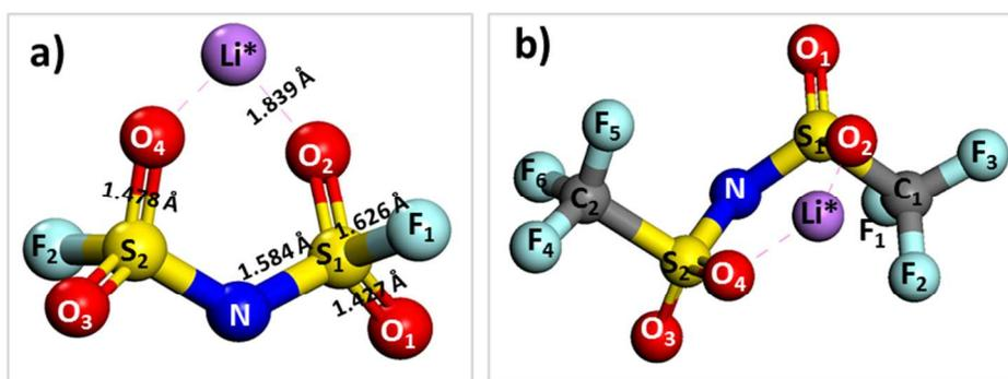
Figure S1. Optimized structures of salt molecules: (a) LiFSI and (b) LiTFSI. Color code as in Figure 1.
