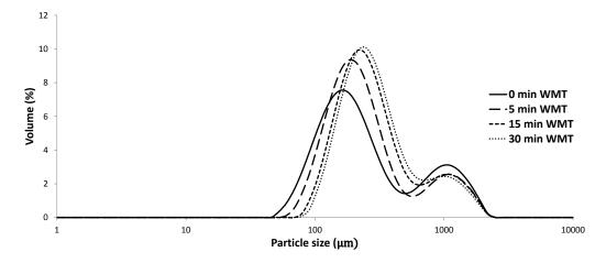
Figure A.7: Granule size distributions produced at 30% LL, 368 rpm and 0-30 min WMT.
