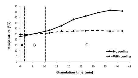
Figure 3.8: Temperature profiles of powder bed throughout the 3 main stages in granulation process. Region A: Pre-mixing, Region B: Liquid addition and Region C: Wet massing
