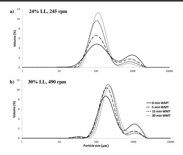
Figure 4.2: Granule size distributions produced at a) 24% LL and 245 rpm and b) 30% LL and 490 rpm narrowed down after 30 min of wet massing.
