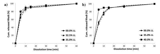
Figure 6.12: Dissolution profiles of "steady state" granules of different formulations: a) 69 wt% lactose and 25 wt% MCC and b) 64 wt% lactose and 30 wt% MCC
