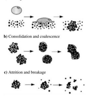
Figure 2.2: Modern approach of describing granulation process as a combination of three sets of rate processes. Adopted from Iveson et al. (2001).
