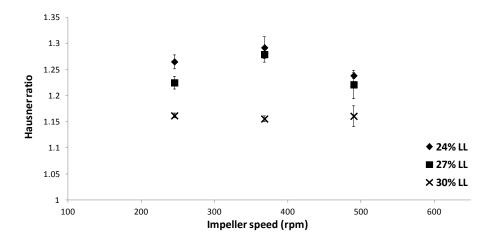
Figure 4.17: Effect of impeller speed on Hausner ratio at different liquid levels.
