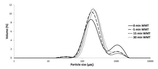
Figure A.10: Granule size distributions produced at 30% LL, 490 rpm and 0-30 min WMT.
