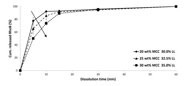
Figure 6.10: Dissolution profiles of "steady state" granules with increasing amount of MCC in formulation and of similar size distributions by adjusting the liquid level.
