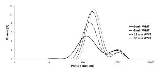
Figure A.4: Granule size distributions produced at 30% LL, 245 rpm and 0-30 min WMT.
