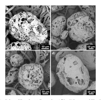
Figure 6.9: Morphology of "steady state" granules: a) 74 wt% lactose and 20 wt% MCC, b) 69 wt% lactose and 25 wt% MCC, c) 64 wt% lactose and 30 wt% MCC and d) 59 wt% lactose and 35 wt% MCC after 60 min of dissolution time.
