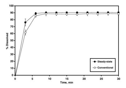
Figure 2.26: Dissolution profiles of tablets compressed from granules produced in "steady state" and "conventional" granulation. Taken from Michaels *et al.* (2009).
