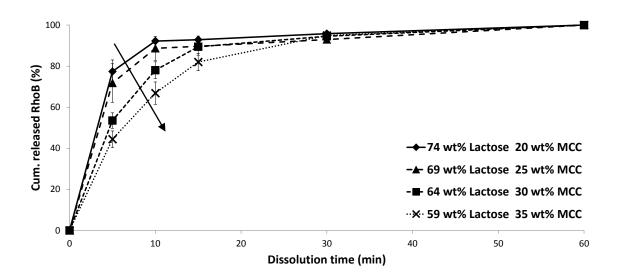
Figure 6.8: Dissolution profiles of "steady state" granules with increasing amount of MCC in formulation, produced at 30% LL and 490 rpm.
