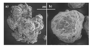
Figure 2.21: Granule morphology changes during wet massing period: a) 0 min WMT and b) 40 min WMT in "steady state" granulation. Taken from Michaels *et al.* (2009).
