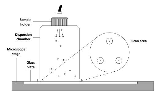
Figure 3.11: "Steady state" granules in the dispersion unit were dispersed on the glass plate.
