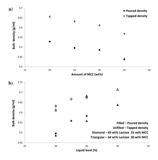
Figure 6.6: a) Effect of formulation on the poured density and tapped density of granules at 30% LL and 490 rpm. b) Effect of liquid level on the poured density and tapped density of granules of different formulations.
