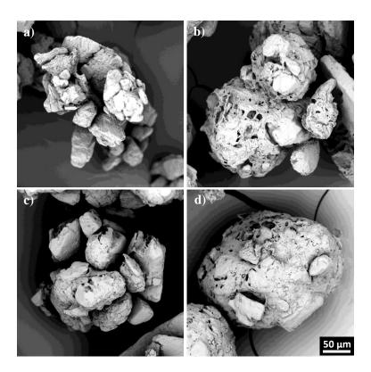
Figure 4.8: Morphology of "steady state" granules produced at a) 24% LL and 245 rpm, b) 30% LL and 245 rpm, c) 24% LL and 490 rpm and d) 30% LL and 490 rpm.
