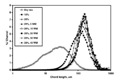
Figure 2.20: The existence of "steady state" condition in HSWG where granule size distribution did not show significant changes towards the end of wet massing period. Taken from Michaels et al. (2009).
