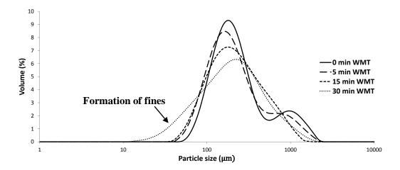
42290Figure 6.13: Size distributions of mannitol-MCC formulated granules produced at 30% LL, 490 rpm and 0-30 min wet massing.
