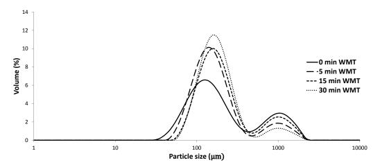
Figure A.6: Granule size distributions produced at 27% LL, 368 rpm and 0-30 min WMT.
