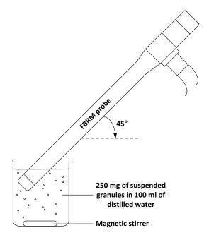
Figure 3.15: FBRM angled at  $45^{\circ}$  and faced the beaker wall to detect the particles in solution.
