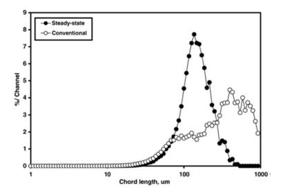
Figure 2.19: Chord-length distributions of wet granules produced by "steady state" granulation and "conventional" granulation at 2-L scale. Taken from Michaels *et al.* (2009).
