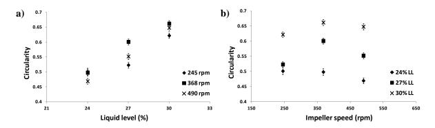
Figure 4.12: Effects of a) liquid level at different impeller speeds and b) impeller speed at different liquid levels on granule circularity after 30 min of wet massing.
