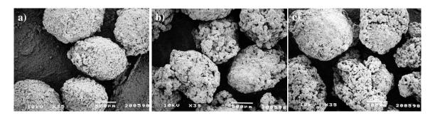
Figure 2.14: Morphology of granules of 1000-1400 μm produced after a) 25 min at 450 rpm, b) after 17 min at 800 rpm and c) after 4 min at 1500 rpm. Taken from Ohno *et al.* (2007).
