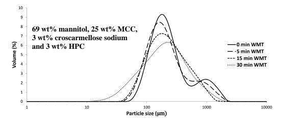
Figure A.13: Granule size distributions produced at 30% LL, 490 rpm and 0-30 min WMT.
