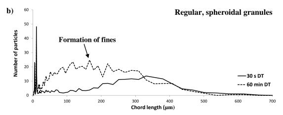
Figure 5.6: FBRM used to detect the change in number of particle during dissolution testing. a) Irregular-shaped granules (24% LL and 245 rpm) and b) Regular, spheroidal granules (30% LL and 490 rpm)
