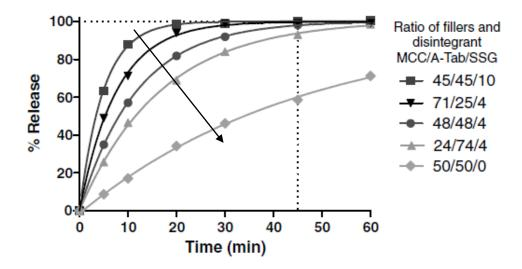
Figure 2.23: Dissolution comparison between different excipient (MCC, calcium dibasic phosphate and disintegrant SSG) ratios and a constant drug load. Inset from am Ende 2011.
