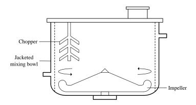
Figure 2.4: Schematic diagram of a high shear mixer granulator.
