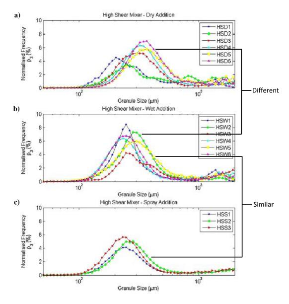
Figure 2.7: Granule size distributions obtained using three different liquid delivery methods: a) Dry addition, b) Wet addition and c) Spray addition in high shear mixer. Taken from Osborne et al. (2011).
