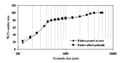
Figure 2.8: Effect of liquid delivery methods on granule size distribution. Taken from Rahmanian *et al.* (2011).
