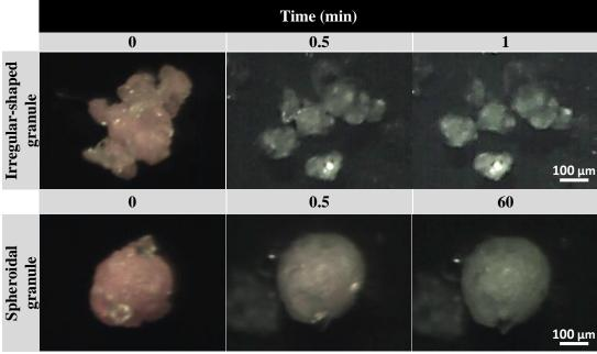
Figure 5.5: Single particle dissolution: 1. Irregular-shaped granules produced at 24% LL and 245 rpm and 2. Regular, spheroidal granules produced at 30% LL and 490 rpm
