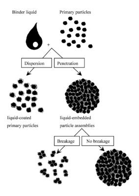
Figure 2.10: Schematic overview of the possible nucleation mechanisms in the high shear mixer granulator. Inset from Dries and Vromans (2004).
