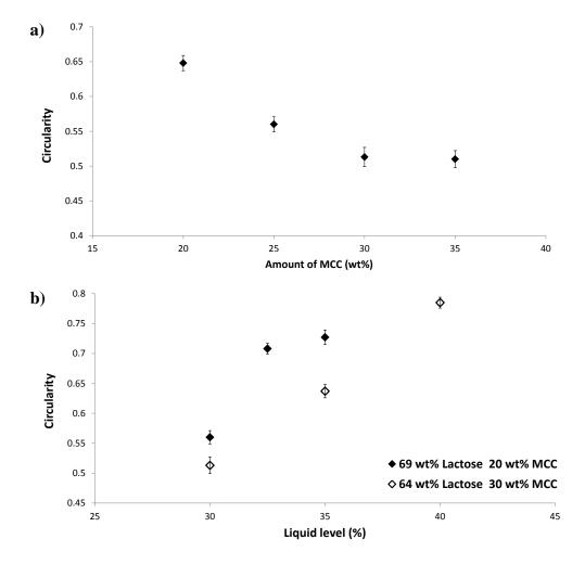
Figure 6.4: a) Effect of formulation on the circularity of granules at 30% LL and 490 rpm. b) Effect of liquid level on the circularity of granules of different formulations.
