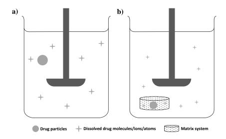
Figure 2.24: Schematic diagram illustrating the differences between the terms: a) "Drug dissolution" and b) "Drug release". Adapted from Siepmann *et al.* (2013).
