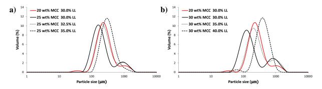
Figure 6.3: Adjustment of liquid level to achieve similar size distribution (74 wt% lactose and 20 wt% MCC). a) 69 wt% lactose and 25 wt% MCC and b) 64 wt% lactose and 30 wt% MCC
