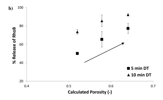
Figure 6.17: Effect of matrix porosity (amount of soluble component) on the release of Rhodamine B within the first 10 min dissolution window. a) Varying composition of formulation (20-35 wt% MCC) with constant liquid level of 30% and b) Varying liquid level (30-35%) at different compositions of formulation (20-30 wt% MCC)
