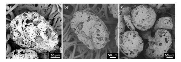
Figure 6.11: Morphology of "steady state" granules: a) 74 wt% lactose and 20 wt% (30% LL) MCC, b) 69 wt% lactose and 25 wt% MCC (32.5% LL) and c) 64 wt% lactose and 30 wt% MCC (35% LL) after 60 min of dissolution time.
