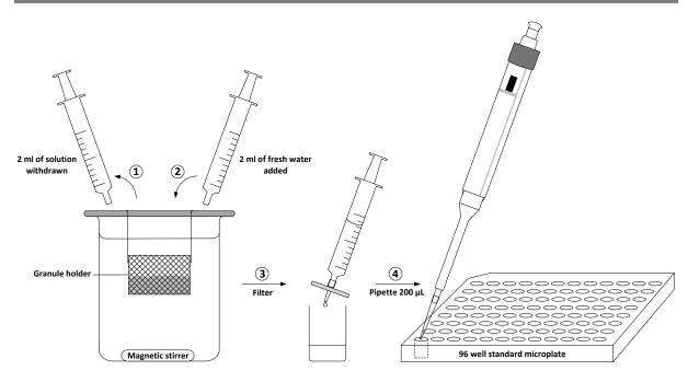
Figure 3.13: Sampling procedure of dissolution test: Step 1. Withdrawal of solution, Step 2: Replenish of fresh deionized water, Step 3. Filter the solution through a syringe filter, Step 4: Pipette the filtered solution into microplate.
