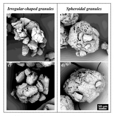
Figure 5.1: Two types of "steady state" granules tested: 1. Irregular-shaped granules – a) 24% LL and 245 rpm, c) 24% LL and 490 rpm and 2. Regular, spheroidal granules – b) 30% LL and 245 rpm, d) 30% LL and 490 rpm.
