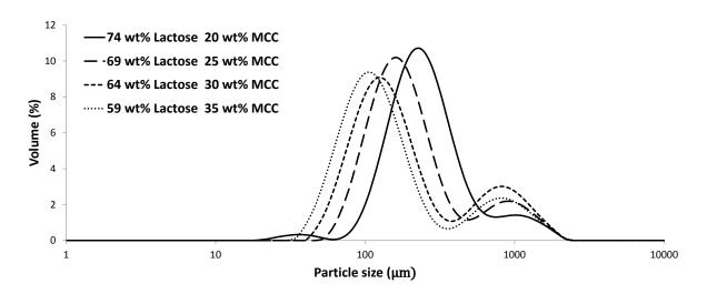
Figure 6.2: Size distributions of "steady state" granules with increasing amount of MCC in formulation, produced at 30% LL and 490 rpm.
