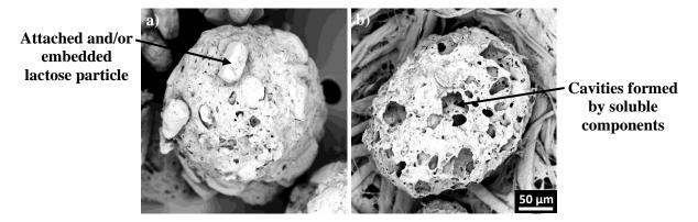
Figure 5.3: Soluble components leached out from "steady state" granules (30% LL and 490 rpm), leaving a matrix of insoluble components. a) 0 min DT and b) 5 min DT
