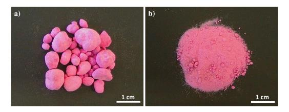
Figure 3.10: Dried granules (at 27% LL, 245 rpm and 0 min WMT) were sieved into two size fractions: a) > 2 mm and b) < 2 mm before being analysed in Mastersizer.
