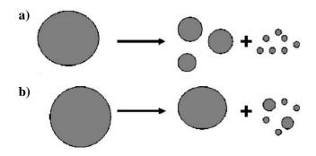
Figure 2.15: Bimodal breakage: a) Many small particles and a few large particles and b) Many small particles and one large particle. Inset from Realpe and Velázquez (2008).
