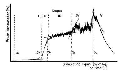
Figure 2.17: Different granulation stages divided up in a power consumption profile at increasing amount of granulating liquid. Taken from Leuenberger *et al.* (2009).
