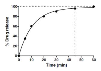
Figure 2.22: "Typical" immediate release dissolution profile, very fast initial release with a levelling off. Inset from am Ende 2011.
