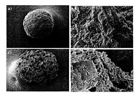
Figure 3.3: a) MCC (Avicel PH101) pellet, b) Surface details of pellet, c) Dissolved MCC (Avicel PH101) pellet and d) Surface details of dissolved pellet. Taken from Kleinebudde (1997).
