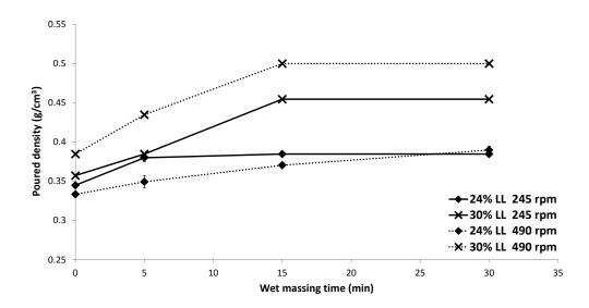
Figure 4.14: Poured density of "steady state" granules over wet massing period.
