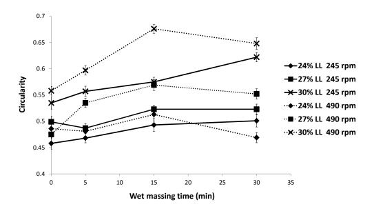
Figure 4.10: Evolution of granule circularity profile during wet massing period at 24-30% LL and 245-490 rpm.
