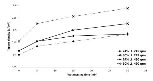
Figure 4.15: Tapped density of "steady state" granules over wet massing period.
