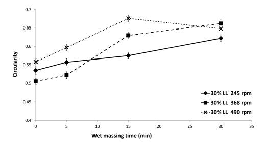
Figure 4.11: Effect of impeller speed on the granule circularity profile at 30% LL.
