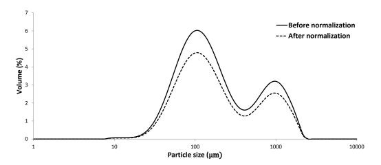
Figure A.1: Normalization of granule size distribution obtained at 24% LL, 245 rpm and 0 min WMT.
