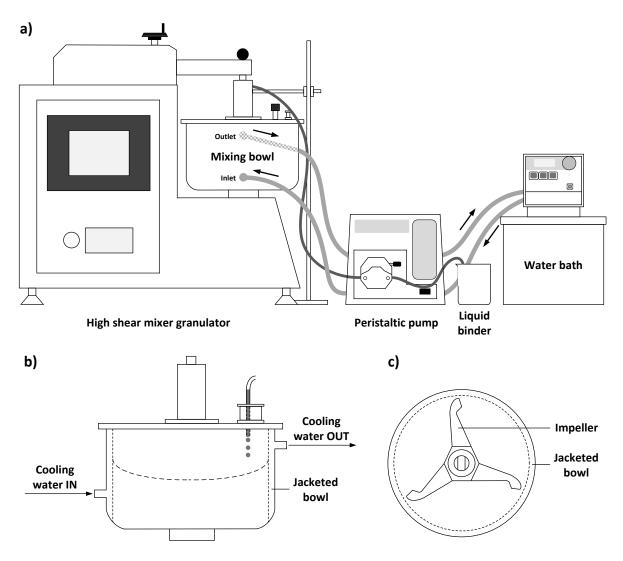
Figure 3.7: a) Experimental setup of "steady state" granulation b) Side view of high shear jacketed mixing bowl c) Impeller 3 blades mounted vertically in mixing bowl
