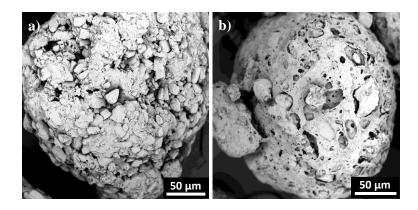
Figure 4.13: "Steady state" granules of 355-500  $\mu m$  formed at a) 24% LL and 245 rpm and b) 30% LL and 490 rpm.
