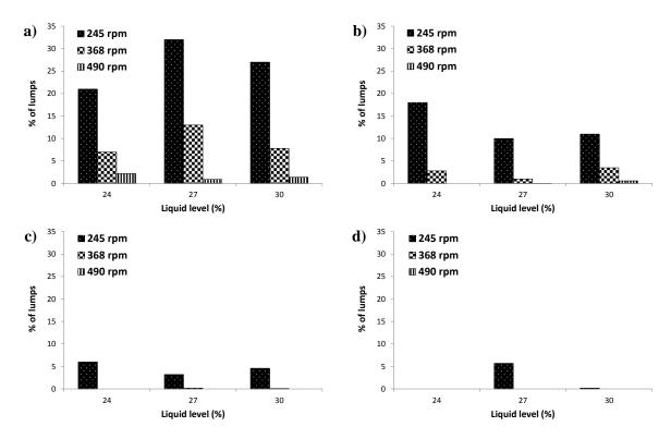
Figure 4.4: Effects of liquid level and impeller speed on the formation and breakage of "lumps" over the wet massing period: a) 0 min WMT, b) 5 min WMT, c) 15 min WMT and d) 30 min WMT.
