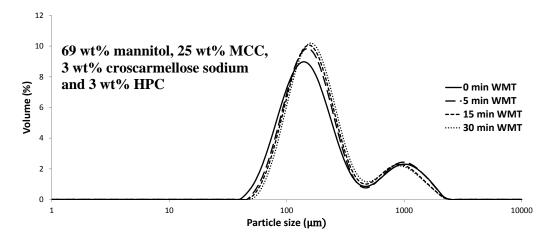
Figure A.11: Granule size distributions produced at 30% LL, 490 rpm and 0-30 min WMT.
