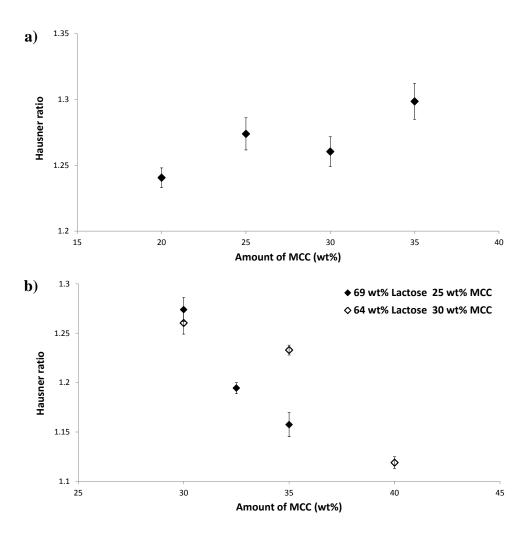
Figure 6.7: a) Effect of formulation on the Hausner ratio at 30% LL and 490 rpm. b) Effect of liquid level on the Hausner ratio of granules of different formulations.
