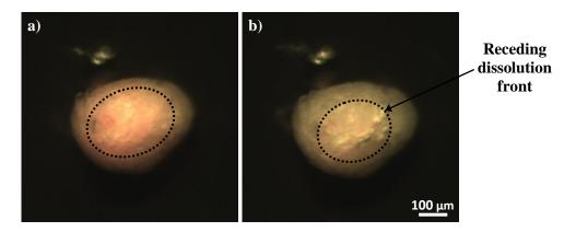
Figure 5.7: Single granule dissolution performed on a granule produced at 30% LL, 490 rpm and after 30 min of wet massing. a) 1 min DT and b) 3 min DT
