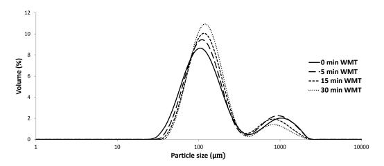
Figure A.8: Granule size distributions produced at 24% LL, 490 rpm and 0-30 min WMT.
