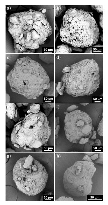
Figure 6.5: Morphology of granules produced at 490 rpm and after 30 min WMT. a) 74 wt% Lactose 20 wt% MCC – 30.0% LL, b) 69 wt% Lactose 25 wt% MCC – 30.0% LL, c) 69 wt% Lactose 25 wt% MCC – 32.5% LL, d) 69 wt% Lactose 25 wt% MCC – 35.0% LL, e) 64 wt% Lactose 30 wt% MCC – 30.0% LL, f) 64 wt% Lactose 30 wt% MCC – 35.0% LL, g) 64 wt% Lactose 30 wt% MCC – 40.0% LL, h) 59 wt% Lactose 35 wt% MCC – 30.0% LL
