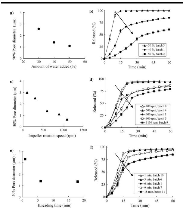
Figure 2.25: Effect of process parameters: a-b) amount of water added, c-d) impeller rotation speed and e-f) kneading time on 50% pore diameter (left) and dissolution profiles of mefenamic acid in tablets (right). Inset from Ohno et al. (2007).
