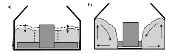
Figure 2.13: Two types of flow regime observed in a high shear granulator: a) Bumping flow and b) Roping flow. Inset from Litster *et al.* (2002).
