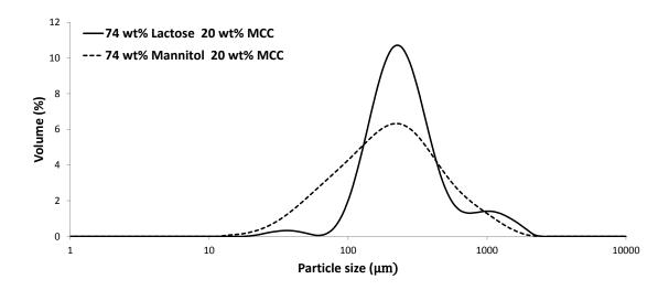
Figure 6.14: Granule size distributions produced using a lactose-MCC formulation and a mannitol-MCC formulation at 30% LL and 490 rpm.
