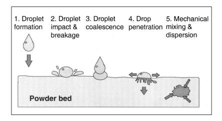
Figure 2.11: The five steps of nucleation: 1. Droplet formation, 2. Droplet impact on the powder and possible breakage, 3. Droplet coalescence at the powder surface, 4. Droplet penetration into the powder pores and 5. Mixing of the liquid and powder by mechanical dispersion. Inset from Litster *et al.* (2001)
