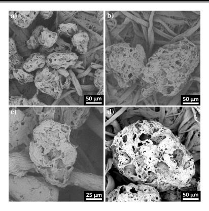
Figure 5.4: Morphology of "steady state" granules produced at a) 24% LL and 245 rpm, b) 30% LL and 245 rpm, c) 24% LL and 490 rpm and d) 30% LL and 490 rpm after 60 min of dissolution time.
