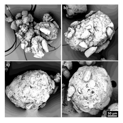
Figure 4.7: Rounding and surface smoothing of "steady state" granules produced at 30% LL and 490 rpm were observed over the wet massing period: a) 0 min WMT, b) 5 min WMT, c) 15 min WMT and d) 30 min WMT.
