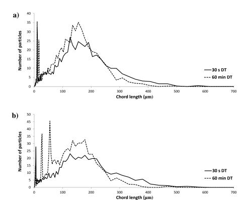
Figure E.1: Evolution of granule size distribution profiles during dissolution testing: a) Run 1 and b) Run 2 for irregular-shaped granules produced at 24% LL and 245 rpm
