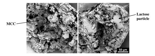
Figure 4.9: Internal structure of "steady state" granules produced at 30% LL and 490 rpm.
