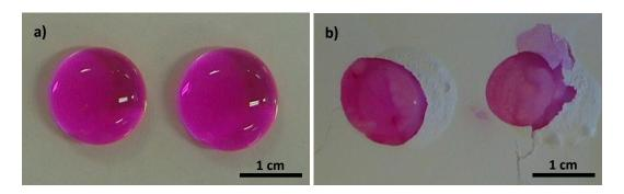
Figure 3.9: a) Liquid droplets that formed after exiting the delivery tube and b) Liquid droplets that fell on lactose powder bed in a petri dish.
