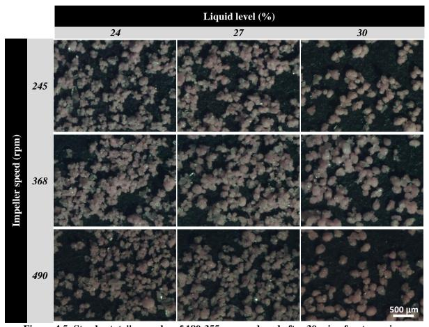
Figure 4.5: Steady state" granules of 180-355 µm produced after 30 min of wet massing.
