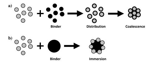
Figure 2.9: Two nucleation mechanisms proposed which take into account the effect of the size of binder droplet: a) Immersion distribution and b) Distribution mechanism. Adapted from Schaefer *et al.* (1996).
