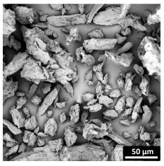
Figure 3.2: Microcrystalline cellulose
