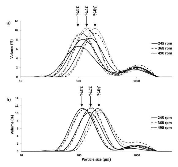
Figure 4.3: Granule size distributions produced a) after 5 min of wet massing and b) at the end of wet massing period at 3 different impeller speeds.
