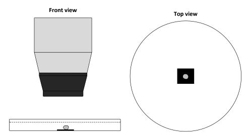
Figure 3.14: A single "steady state" granule dissolved in a petri dish and examined under optical microscope.
