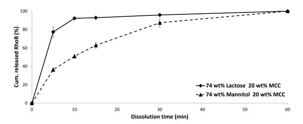
Figure 6.15: Dissolution profiles of lactose-MCC formulated and mannitol-MCC formulated "steady state" granules.
