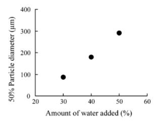
Figure 2.5: Effect of amount of liquid on 50% particle diameter at an impeller rotation speed of 600 rpm and wet massing time of 6 min. Taken from Ohno *et al.* (2007).
