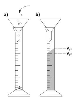
Figure 3.12: a) "Steady state" granules poured into a 5 ml graduated measuring cylinder through a funnel. b) Poured volume was determined by taking the average of  $V_{p1}$  and  $V_{p2}$ .
