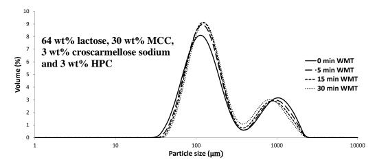
Figure A.12: Granule size distributions produced at 30% LL, 490 rpm and 0-30 min WMT.
