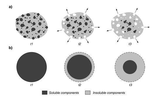
Figure 5.8: a) Leaching mechanism occurs during dissolution of "steady state" granules b) Shrinking core model proposed to describe the leaching mechanism (where t3>t2>t1)
