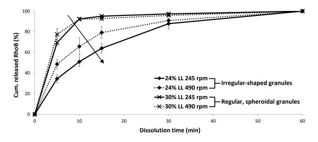
Figure 5.2: Dissolution profiles of "steady state" granules (180-355  $\mu$ m) produced after 30 min of wet massing) obtained by monitoring the release of Rhodamine B over time.
