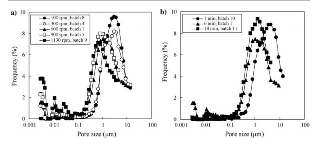
Figure 2.16: Effects of a) impeller rotation speed and b) wet massing time on pore size distribution. Taken from Ohno *et al.* (2007).
