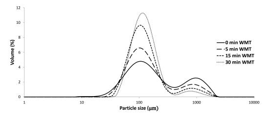
Figure A.2: Granule size distributions produced at 24% LL, 245 rpm and 0-30 min WMT.
