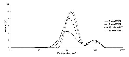
Figure A.3: Granule size distributions produced at 27% LL, 245 rpm and 0-30 min WMT.
