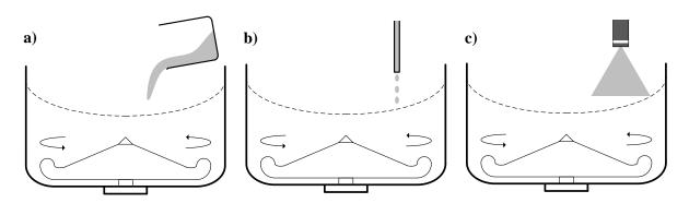
Figure 2.6: Different methods of liquid delivery: a) Pouring, b) Dripping and c) Spraying.
