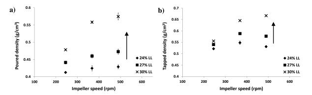
Figure 4.16: Effect of impeller speed on a) poured and b) tapped densities of "steady state" granules at different liquid level.
