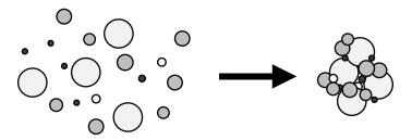
Figure 2.1: Fine particles are agglomerated into larger entity called granule.
