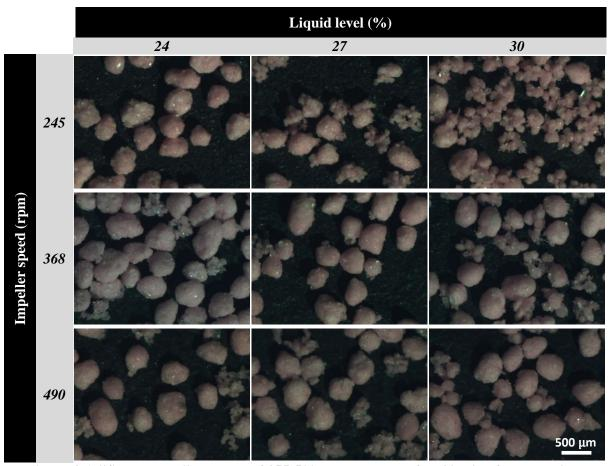
Figure 4.6: "Steady state" granules of 355-500 µm produced after 30 min of wet massing.
