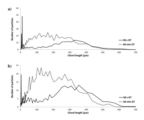
Figure E.2: Evolution of granule size distribution profiles during dissolution testing: a) Run 1 and b) Run 2 for regular, spheroidal granules produced at 30% LL and 490 rpm
