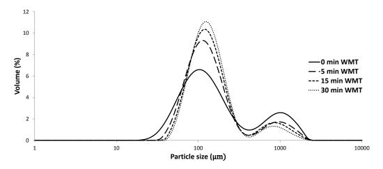
Figure A.5: Granule size distributions produced at 24% LL, 368 rpm and 0-30 min WMT.
