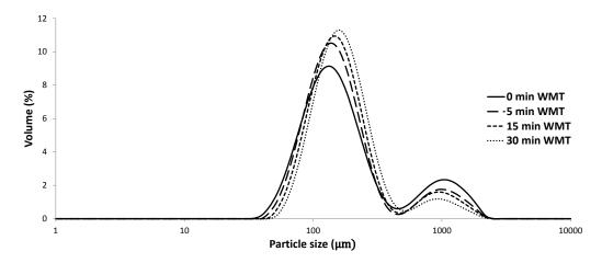
Figure A.9: Granule size distributions produced at 27% LL, 490 rpm and 0-30 min WMT.
