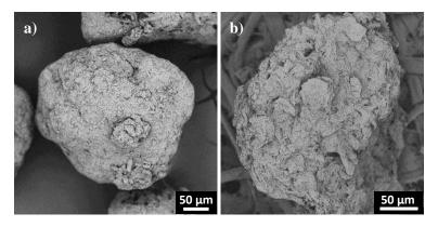
Figure 6.16: Morphology of mannitol-MCC formulated granules a) before and b) after 60 min of dissolution testing.
