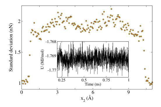
Figure S5 – Standard deviation of mean force calculation using FEP for sliding of unfrozen case along the  $x_2$  direction. The inset shows the potential energy during the sampling at  $x_2 = 10.5$ Å.
