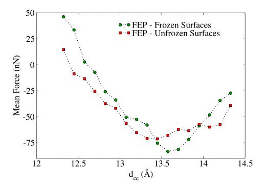
Figure S2 – A comparison between the FTF mean force for frozen and unfrozen cases below the distance of one layer of water.
