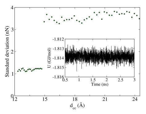
Figure S3 – Standard deviation of mean force calculation using FEP for FTF case. The inset shows the potential energy during the sampling at  $d_{cc} = 13.5$ Å.
