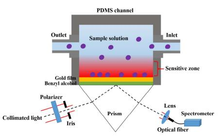
Figure S1. Schematic diagram of home-built spectral Surface Plasmon Resonance (SPR)
