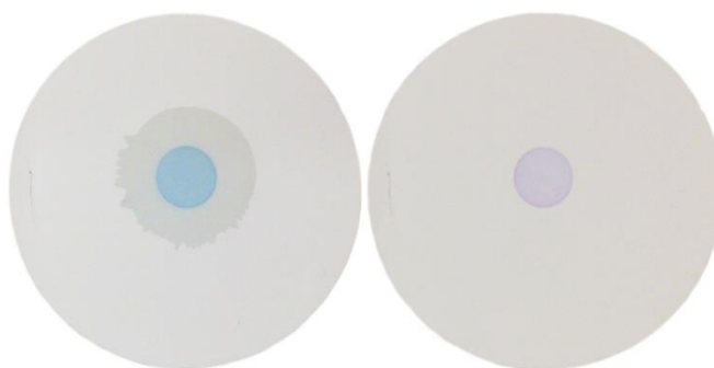
Figure S6. Pictures showing the color changes of chromoionophore I and NaTFPB mixture on a nylon filter paper under different conditions: (left): adding a drop of water; (right): after the water evaporated.
