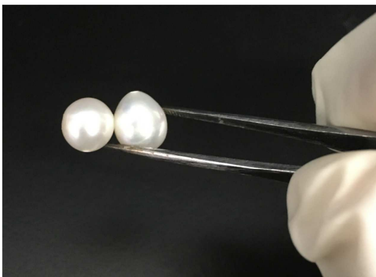
Figure S13. By using 200 \mu\text{L} of DDDEKC-PAMAM solution (2.25 mg/mL), pearls (8 mm in diameter) were stucked. It indicates that the DDDEKC-PAMAM coating has a strong binding force on the surface of biominerals.
