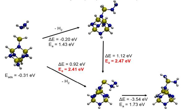
Scheme S2. Diamination reaction pathway of hydrazine onto the silylated nitride surface.
