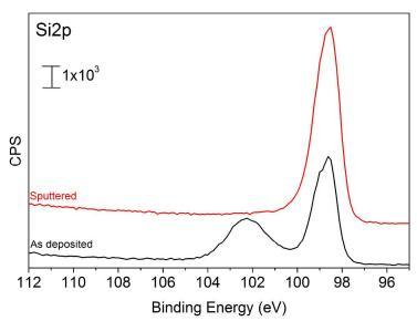
**Figure S2.** High resolution Si2p XPS spectra of the film as deposited and after being fully removed by 3 kV Ar<sup>+</sup> ion sputtering.
