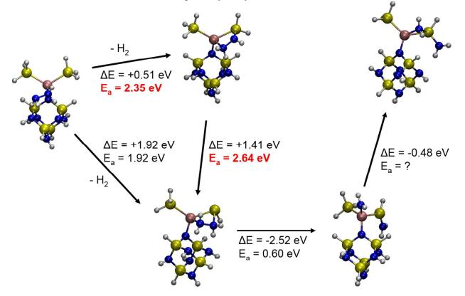
Scheme S4. Monoamination reaction pathway of hydrazine onto the aluminum-activated surface.
