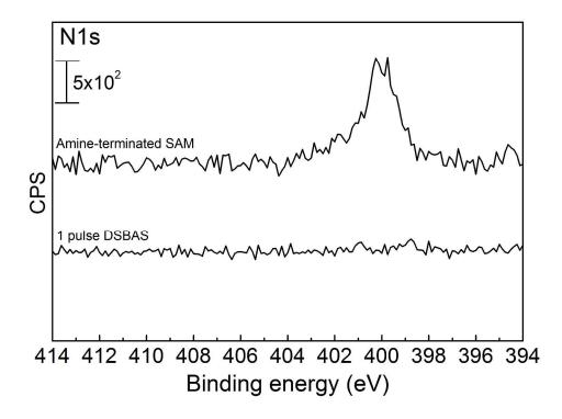
Figure S1. N1s XPS spectra of an amine-terminated SAM and OH-terminated silicon following 1 pulse of DSBAS.
