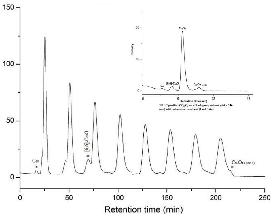
**Figure S14.** Recycling HPLC profile of C<sub>60</sub>O<sub>2</sub> on a Buckyprep-M column (10 × 250 mm) with toluene as the eluent (5 mL/min)
