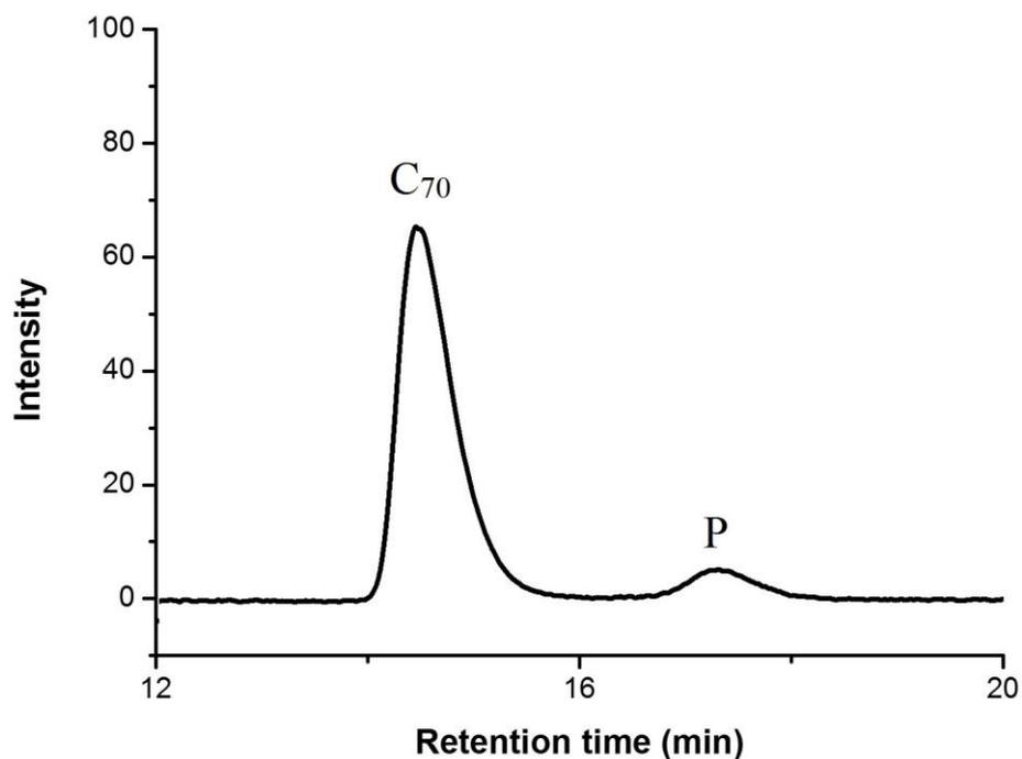
**Figure S19.** HPLC profile of C<sub>70</sub> treated with plasma jet (Ar: 200 mL/min, O<sub>2</sub>: 400 mL/min, 3.5 kV, -10 °C, 15 min) on a Buckyprep column (4.6 × 250 mm) with toluene as the eluent (1 mL/min)
