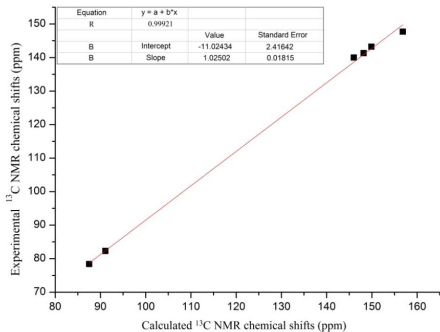
**Figure S16.** Linear correlation between experimental<sup>1</sup> and GIAO (B3LYP/6-311+ G (2df, 2pd)) calculated <sup>13</sup>C NMR data for *cis*-1 isomer of C<sub>60</sub>O<sub>2</sub>:  $\delta_{(\text{exp})} = 1.02502\delta_{(\text{cal})} - 11.02434$  (R = 0.99921)
