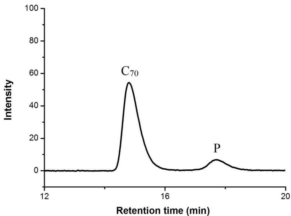
**Figure S18.** HPLC profile of C<sub>70</sub> treated with plasma jet (Ar: 200 mL/min, O<sub>2</sub>: 400 mL/min, 3.5 kV, 0 °C, 30 min) on a Buckyprep column (4.6 × 250 mm) with toluene as the eluent (1 mL/min)
