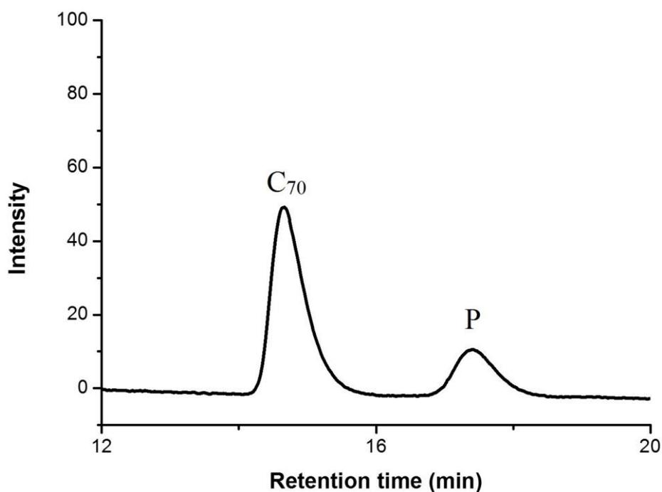
**Figure S17.** HPLC profile of C<sub>70</sub> treated with plasma jet (Ar: 200 mL/min, O<sub>2</sub>: 400 mL/min, 3.5 kV, 0 °C, 15 min) on a Buckyrep column (4.6 × 250 mm) with toluene as the eluent (1 mL/min)
