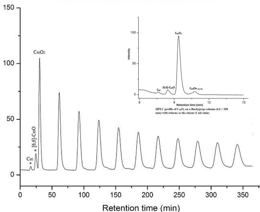
**Figure S13.** Recycling HPLC profile of C<sub>60</sub>O<sub>2</sub> on a Buckyprep column (10 × 250 mm) with toluene as the eluent (5 mL/min)
