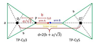
**Scheme S1**. Theoretical estimation of the distance between TP-Cy3 and TP-Cy5 when FRET. Scheme represent the top view of the assembly of TP-Cy3 (red) and TP-Cy5(blue).
