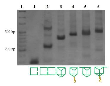
**Figure S2.** N-PAGE (5%) results of self-assembly of DNA nanoprisms, run at 20 V for 4 h. Lanes 1-3 show the stepwise assembly of DNA nanoprism scaffold, demonstrating that the 3D scaffold was the major product finally shown with a single band in lane 3. Lanes 4-6 represent this scaffold loading a cholesterol-labeled DNA anchor on the bottom face, an overhang DNA arm on the top face, and both sequences on both faces, respectively. The gels were imaged using a Bio-Rad ChemiDoc XRS System.
