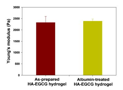
**Figure S11.** Comparison of Young's moduli between as-prepared and albumin-treated HA-EGCG hydrogels tested in this study. HA-EGCG hydrogels were formed at the optimized concentrations of HRP (0.24 units mL<sup>-1</sup>) and H<sub>2</sub>O<sub>2</sub> (0.76 mM). For albumin treatment, hydrogel disks were immersed in 2 mL of PBS (pH 7.4) containing bovine serum albumin (100 mg mL<sup>-1</sup>) for 72 h at 37°C. All the results are expressed as mean  $\pm$  SD (n = 3).
