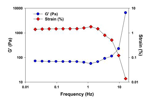
**Figure S8.** Evolution of the storage modulus (G') and strain of HA-EGCG hydrogel as a function of applied frequency of oscillatory shear stress. HA-EGCG hydrogel was formed at the optimized concentrations of HRP (0.24 units mL<sup>-1</sup>) and  $H_2O_2$  (0.76 mM).
