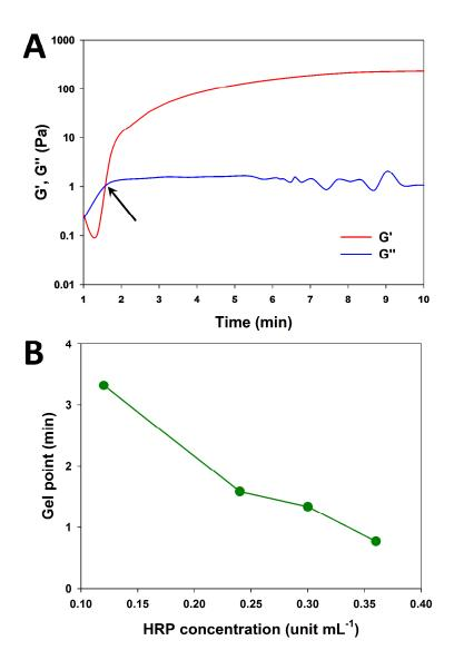
**Figure S7.** (A) Time course of changes in the storage modulus (G', red curve) and loss modulus (G'', blue curve) of HA-EGCG hydrogel formed at the optimized concentrations of HRP (0.24 units mL<sup>-1</sup>) and  $H_2O_2$  (0.76 mM). The arrow indicates the gel point at which the crossover of G' and G'' occurs. (B) Gel points of HA-EGCG hydrogels formed at various concentrations of HRP. The final concentration of  $H_2O_2$  was fixed at 0.76 mM.
