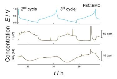
**Figure S5.** Charge-discharge profiles (blue) for the 2nd and 3rd cycles of a Si half-cell with higher loading (~0.4 mg<sub>Si</sub> cm<sup>-2</sup>) using 1 M LiPF<sub>6</sub> in FEC:EMC with the corresponding background corrected mass signals (brown) m/z = 2 (H<sub>2</sub>) and 44 (CO<sub>2</sub>).
