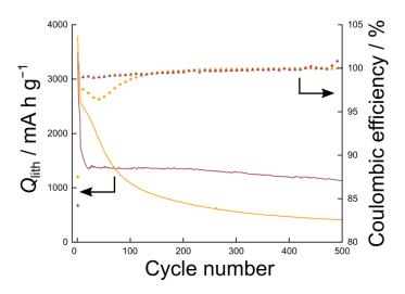
**Figure S1.** Specific lithiation capacities and Coulombic efficiencies for a Si half-cell with higher loading (~0.8  $mg_{Si}$  cm<sup>-2</sup>) using 1 M LiPF<sub>6</sub> in EC:EMC (orange) and FEC:EMC (red).
