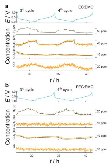
**Figure S3.** Charge-discharge profiles (blue) for the 3rd and 4th cycles of Si half-cells using (a) 1 M LiPF<sub>6</sub> in EC:EMC and (b) FEC:EMC with the corresponding mass signals (brown) m/z = 2 (H<sub>2</sub>), 26 (C<sub>2</sub>H<sub>4</sub>), and 44 (CO<sub>2</sub>), and IR absorption curves (orange) for C<sub>2</sub>H<sub>4</sub>, CO<sub>2</sub>, and CO.
