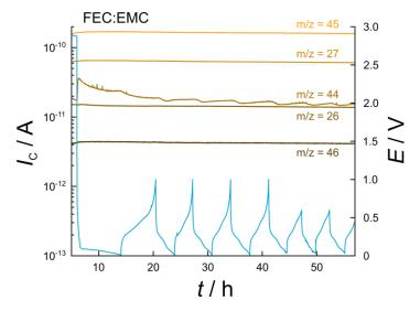
**Figure S2.** Charge-discharge profiles (blue) for the first seven cycles of a Si half-cell using 1 M LiPF<sub>6</sub> in FEC:EMC with the corresponding ion currents (orange/brown) for the main fragments of  $C_2H_3F$ .
