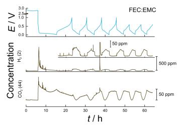
**Figure S4.** Charge-discharge profiles (blue) for the first seven cycles of a Si half-cell with higher loading (~0.4 mg<sub>Si</sub> cm<sup>-2</sup>) using 1 M LiPF<sub>6</sub> in FEC:EMC with the corresponding background corrected mass signals (brown) m/z = 2 (H<sub>2</sub>) and 44 (CO<sub>2</sub>).
