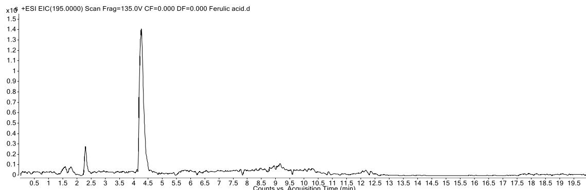
**Figure S51.** Extracted-ion chromatogram of ferulic acid ( $M= 194$  g/mol) in positive ion mode identified by  $[M+H]^+$  m/z 195
