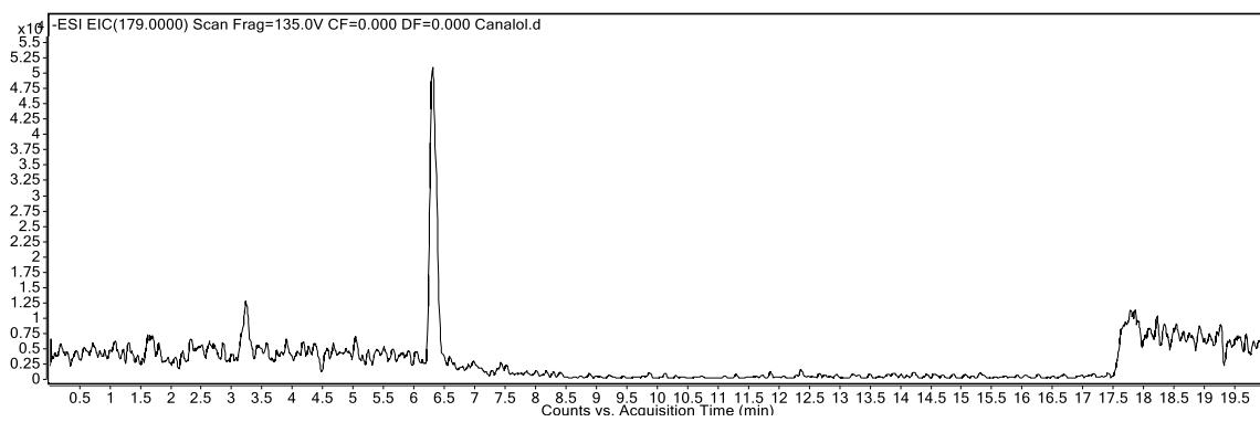
**Figure S56.** Extracted-ion chromatogram of 4-vinylsyringol ( $M= 180$  g/mol) in negative ion mode identified by  $[M-H]^-$  m/z 179
