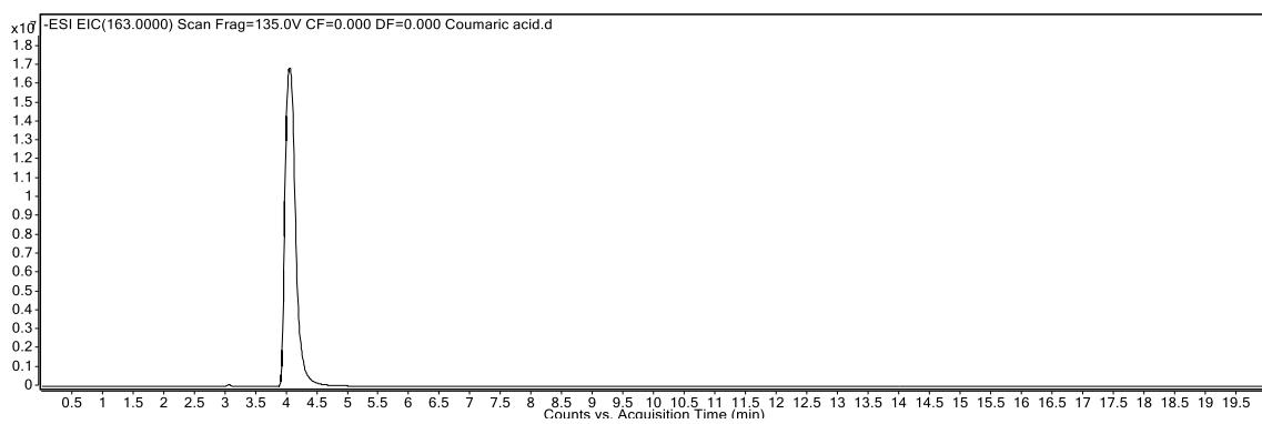
**Figure S48.** Extracted-ion chromatogram of p-coumaric acid ( $M = 164$  g/mol) in negative ion mode identified by  $[M-H]^-$  m/z 163
