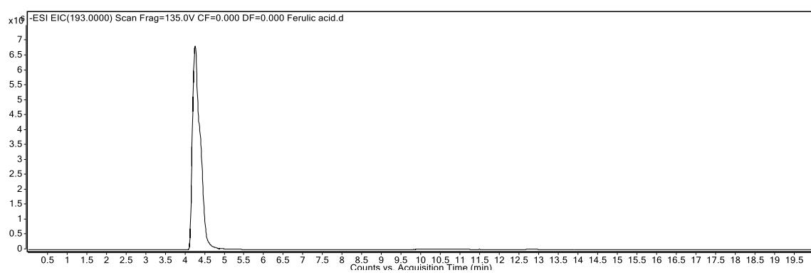
**Figure S52.** Extracted-ion chromatogram of ferulic acid ( $M= 194$  g/mol) in negative ion mode identified by  $[M-H]^-$  m/z 193
