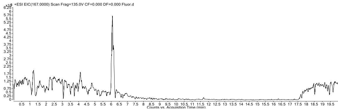
**Figure S35.** Extracted-ion chromatogram of 4-fluorocinnamic acid ( $M= 166$  g/mol) in positive ion mode identified by  $[M+H]^+$  m/z 167
