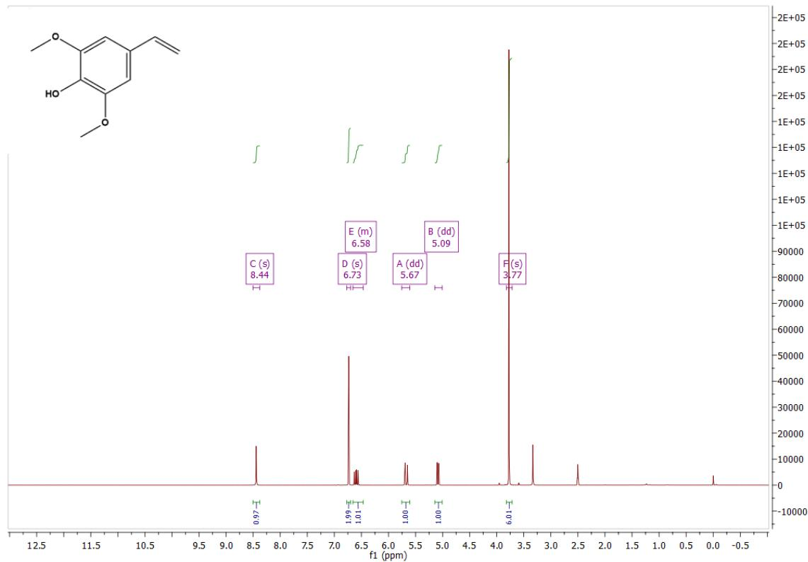
**Figure S53.**  $^1\text{H}$  NMR spectrum of 4-vinylsyringol 4a
