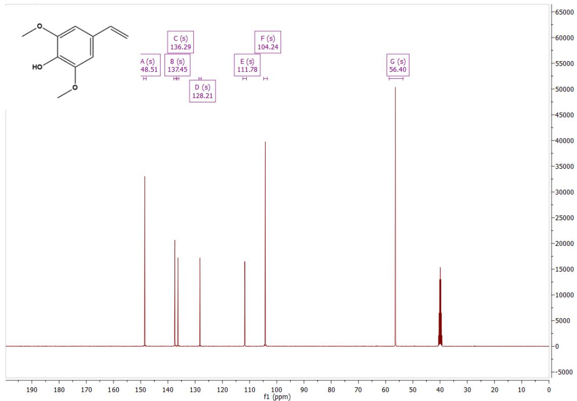
**Figure S54.**  $^{13}\text{C}$  NMR spectrum of 4-vinylsyringol 4a
