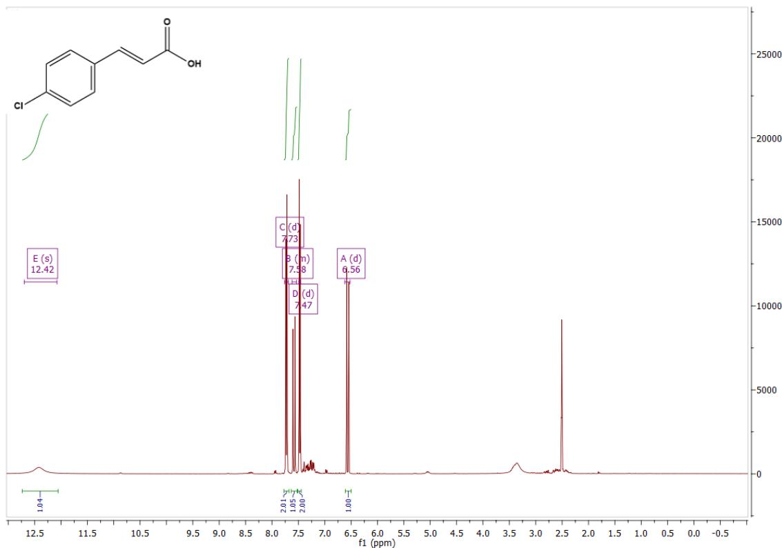
**Figure S37.**  $^1\text{H}$  NMR spectrum of 4-chlorocinnamic acid **3h**
