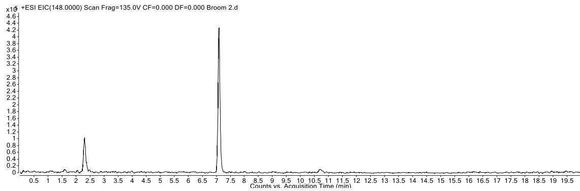
**Figure S43.** Extracted-ion chromatogram of 4-bromocinnamic acid ( $M= 226$  and  $228$  g/mol) in positive ion mode identified by  $[M-\text{Br}^+]$  m/z 148
