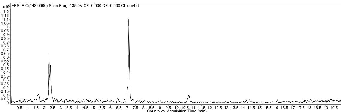
**Figure S39.** Extracted-ion chromatogram of 4-chlorocinnamic acid ( $M= 182$  and  $184$  g/mol) in positive ion mode identified by  $[M-\text{Cl}]^+$  m/z 148
