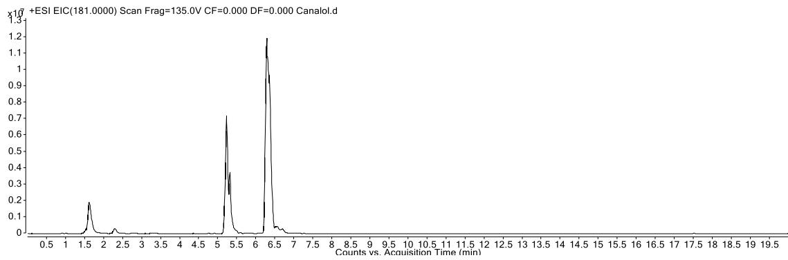
**Figure S55.** Extracted-ion chromatogram of 4-vinylsyringol ( $M= 180$  g/mol) in positive ion mode identified by  $[M+H]^+$  m/z 181
