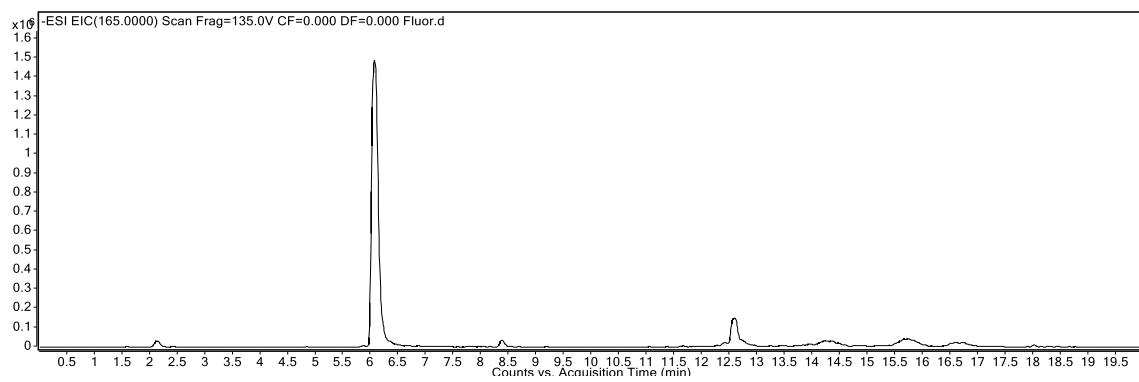
**Figure S36.** Extracted-ion chromatogram of 4-fluorocinnamic acid ( $M= 166$  g/mol) in negative ion mode identified by  $[M-H]^-$  m/z 165
