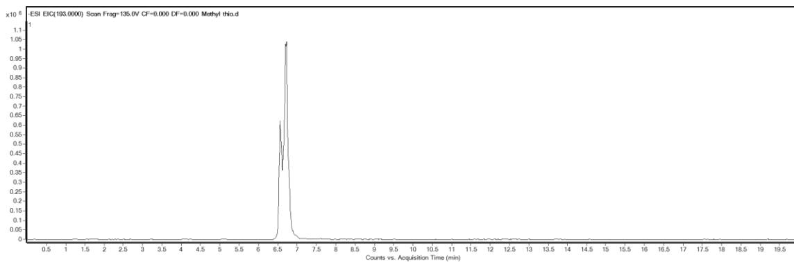
**Figure S32.** Extracted-ion chromatogram of 4-(methylthio)cinnamic acid ( $M= 194$  g/mol) in negative ion mode identified by  $[M-H]^-$  m/z 193
