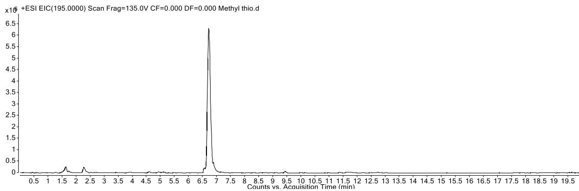
**Figure S31.** Extracted-ion chromatogram of 4-(methylthio)cinnamic acid ( $M= 194$  g/mol) in positive ion mode identified by  $[M+H]^+$  m/z 195
