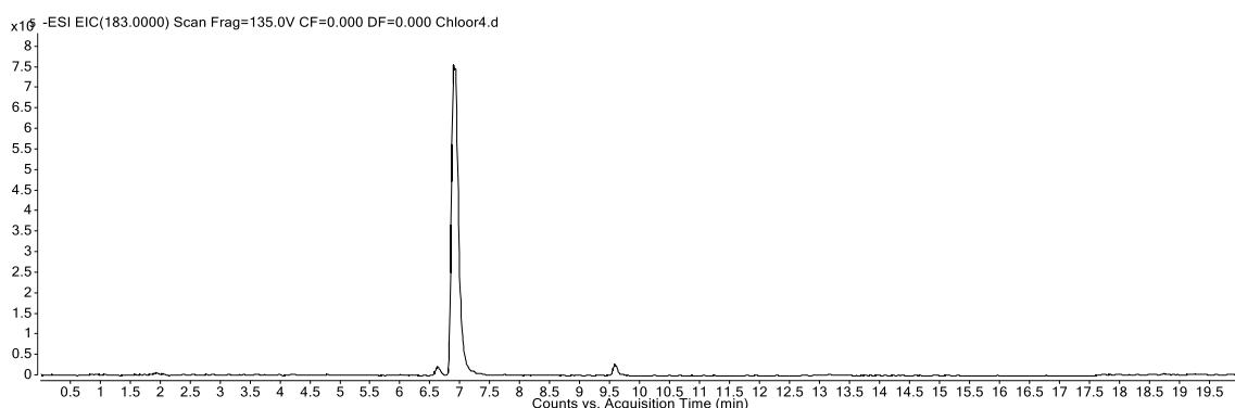
**Figure S40.** Extracted-ion chromatogram of 4-chlorocinnamic acid ( $M= 182$  and  $184$  g/mol) in negative ion mode identified by  $[M-\text{H}]^-$  m/z 181 and 183
