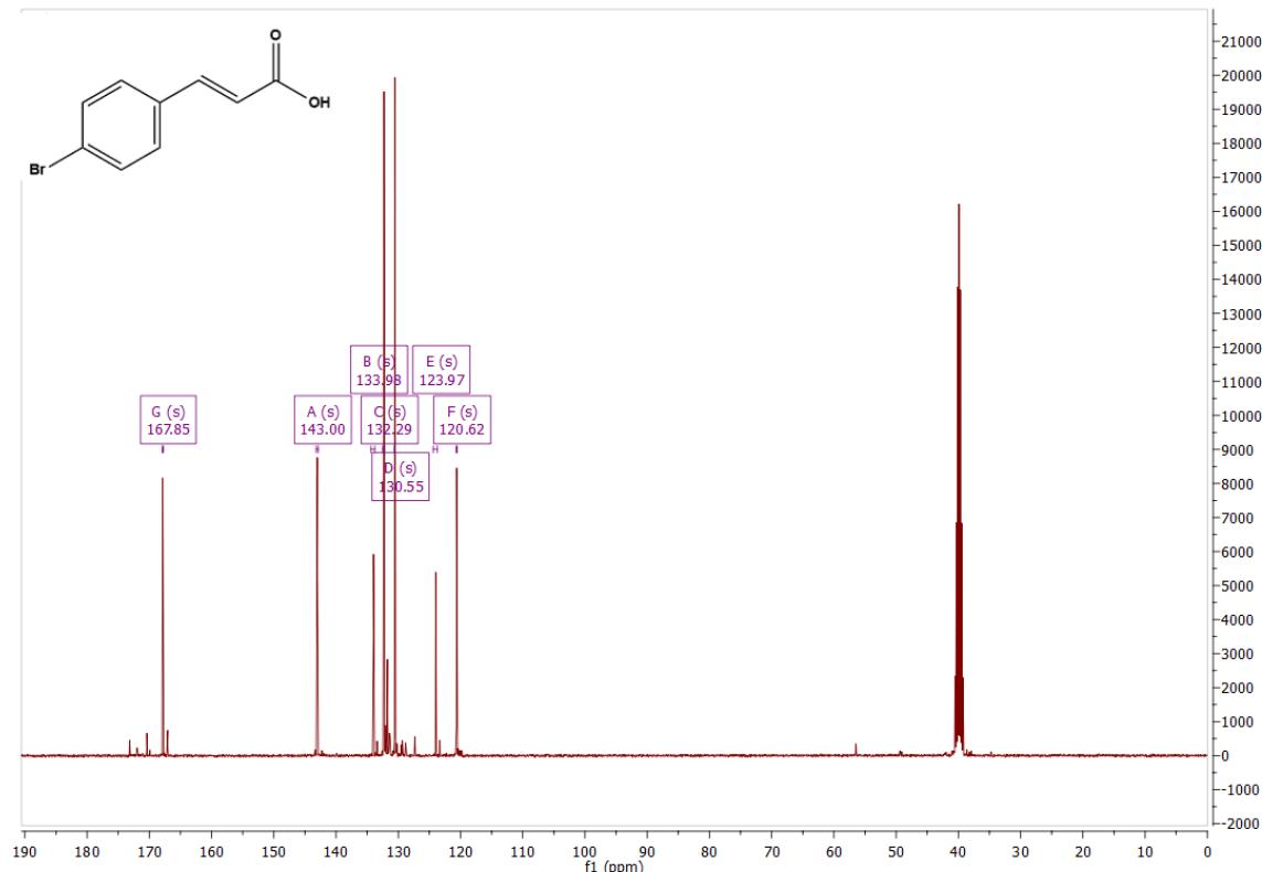
**Figure S42.**  $^{13}\text{C}$  NMR spectrum of 4-bromocinnamic acid **3i**
