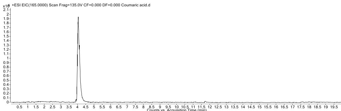
**Figure S47.** Extracted-ion chromatogram of p-coumaric acid ( $M = 164$  g/mol) in positive ion mode identified by  $[M+H]^+$  m/z 165
