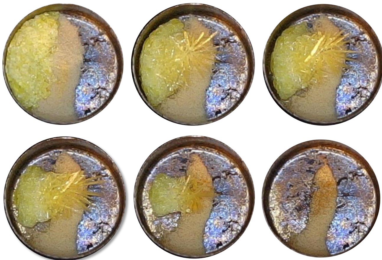
Figure S3: Micrographs of a mixture of 2-hydroxy-1,4-naphthoquinone, 2-hydroxybenzoic acid and anthracene-9,10-dione, showing crystal formation during heating to 300 °C
