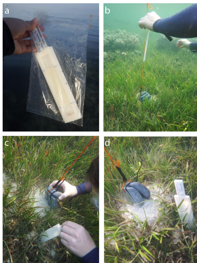
Figure S2. Deployment of sulphide sensitive DGT gels in situ . (a) The sulphide sensitive DGT gels were mounted in DGT samplers. (b) The study site within the seagrass meadow (Green Island, Cairns, Australia). (c) DGT gel deployment. (d) Gel sampler positioned within the seagrass meadow. To enable DGT deployment, a less densely vegetated spot was selected within the dense multi-species seagrass meadow. The DGTs were deployed at sunrise and retrieved at sunset for the daytime measurements and vice versa for the night measurements. Two deployments were performed in the investigated seagrass meadow.
