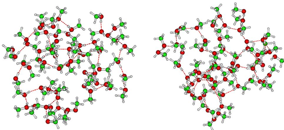
**Figure 1:** Composition of the 62 MeOH (left) and the 54 MeOH + 8 H<sub>2</sub>O (right) clusters used in the force-field parameter assessment.
