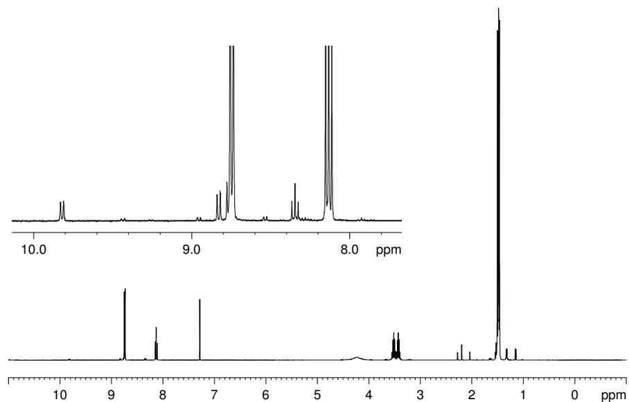
**Figure 4:** NMR spectrum of *iPr*-BTP in pure  $\text{CDCl}_3$  at a concentration of 30 mM. The expansion shows the Signals of minor species in the aromatic region.
