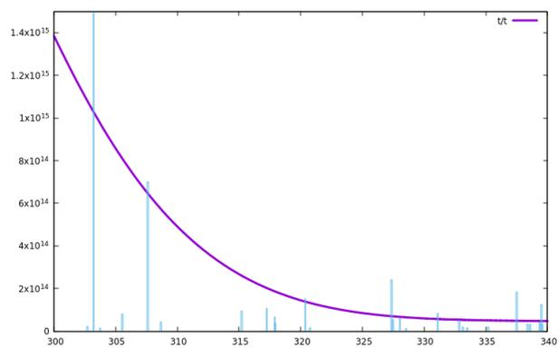
**Figure 2:** Calculated excitations in the 300 to 340 nm region calculated from the 50 MD snapshots MeOH:H<sub>2</sub>O 1:1, t/t conformer.
